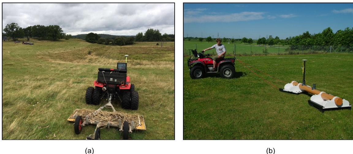
**Figure 3.** Survey configuration of: (a) the three-dimensional ground penetrating radar (3D-GPR) instrument and (b) the DUALEM-21S sensor.
