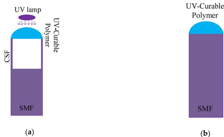
Figure 20. The description of the structures: (a) The lensed fiber consists of SMF, CSF, and UV-curable polymer [90]; (b) Sensor consists of SMF and UV-curable polymer [91].
