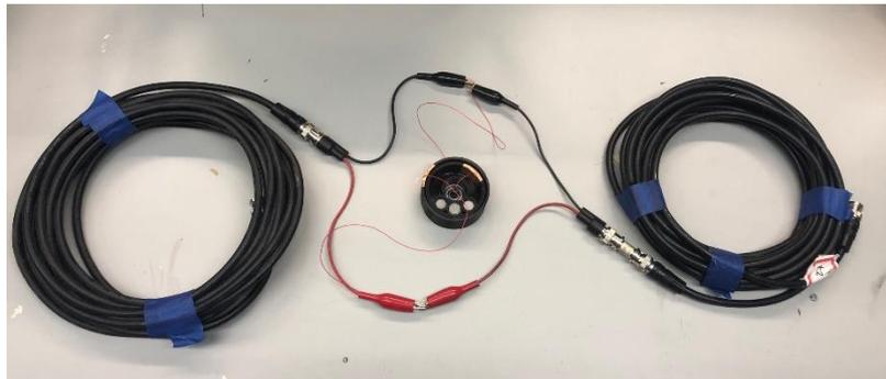
**Figure 7.** The tilt sensor is connected as part of a transmission line setup using RG-6 coaxial cables.
