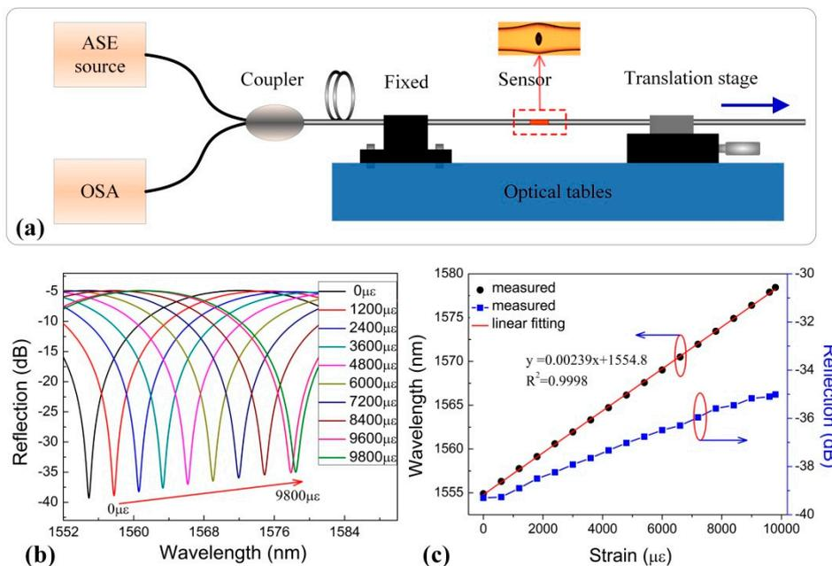
**Figure 3.** (a) Experimental setup for strain measurement. (b) Wavelength shift of interference fringe around  $1555 \text{ nm}$  as a function of tensile strain applied to the air-cavity-based FPI sample. (c) Reflection spectrum evolution of the air-bubble-based FPI sample while the tensile strain increasing from  $0$  to  $9800 \mu\epsilon$ .
