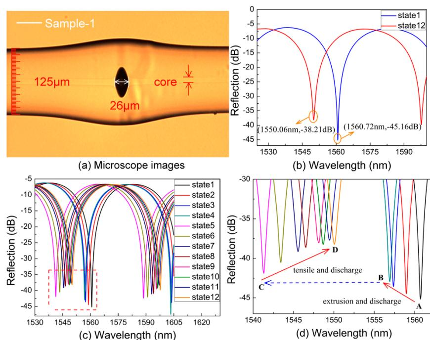
**Figure 1.** (a) Microscope images of the in-fiber Fabry–Perot interferometers (FPI) with a cavity length of 26  $\mu\text{m}$ . (b) The reflection original spectrum and the final spectrum. (c) The dip wavelength of reflection spectra at the same arc discharge states (state 1–12). (d) Enlarged the view of the dotted box.
