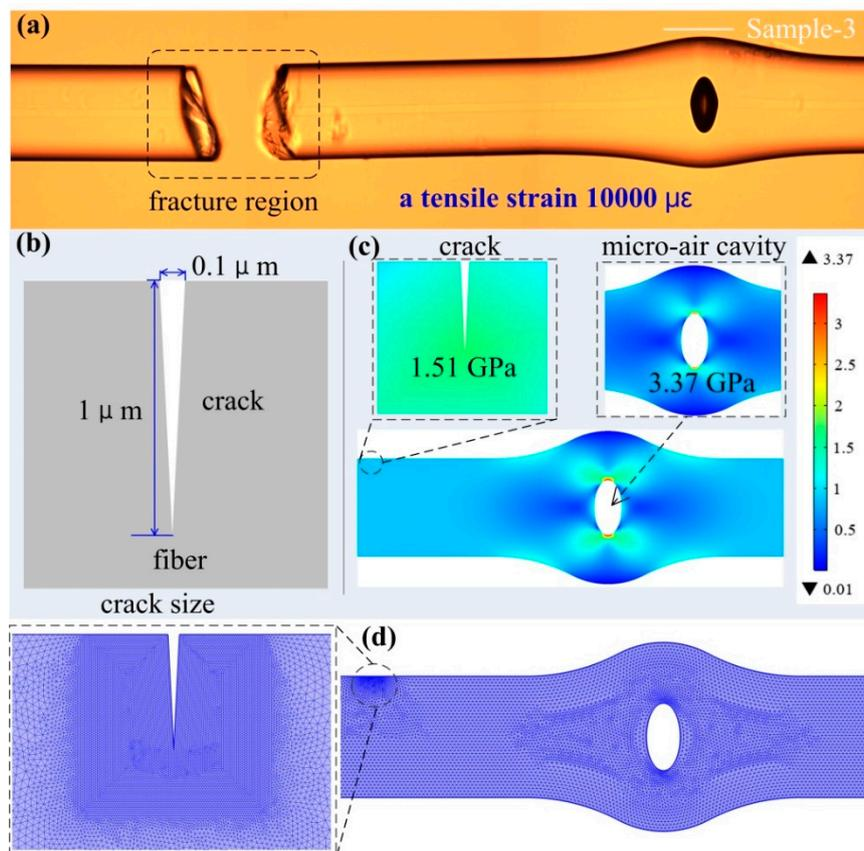
**Figure 4.** (a) Microscope images of the in-fiber FPI with fracture surface appears in the fiber. (b) Geometric model of crack in-fiber. (c) Two-dimensional stress contours while the axial strain of 10,000  $\mu\epsilon$  applied to the model. (d) Mesh of the in-fiber FPI model.
