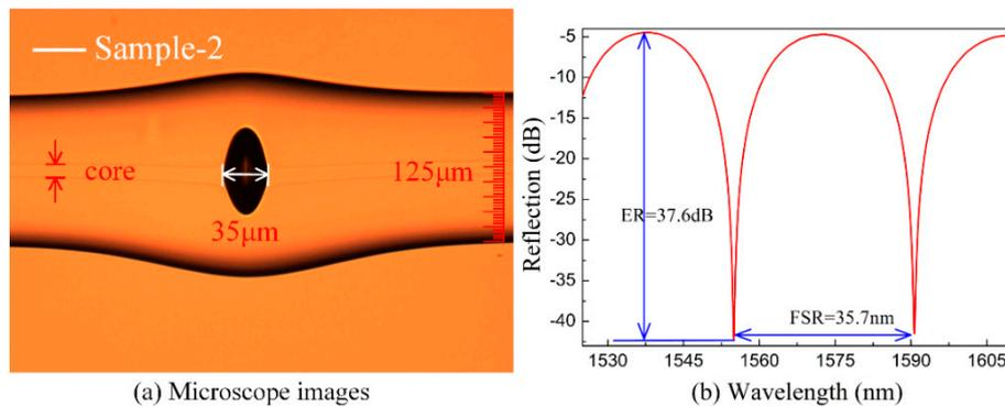
**Figure 2.** (a) Microscope images of the in-fiber FPI with a cavity length of  $\sim 35 \mu\text{m}$ . (b) The corresponding reflection spectrum of the FPI, free spectral range (FSR)  $\sim 35.7 \text{ nm}$ , ER  $\sim 37.6 \text{ dB}$ .
