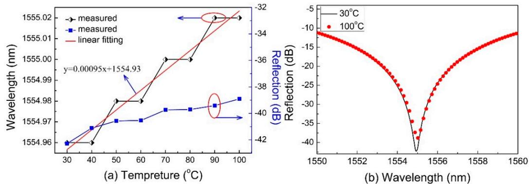
**Figure 5.** (a) Linear relationship between the wavelength shift of the interference dip at  $\sim 1555 \text{ nm}$  and ambient temperature. (b) The reflection spectra of FPI at  $30^\circ\text{C}$  and  $100^\circ\text{C}$ .
