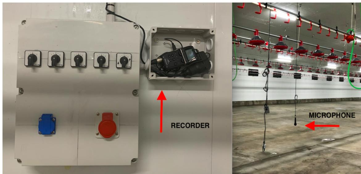
**Figure 2.** Acoustic equipment deployment in the farm H1. On the left, the recorder location. On the right, the microphone hanging from the ceiling in order to avoid physical interaction with the birds.
