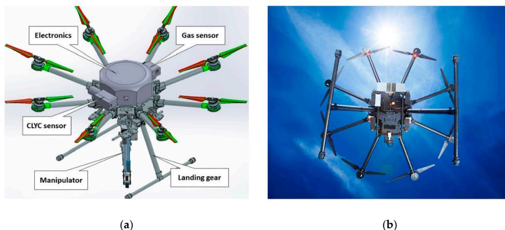
**Figure 1.** (a) Rendering of the unmanned aerial system (UAS) with attached payload; (b) aerial robotic platform in flight.
