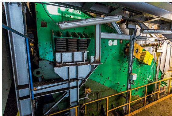
Figure 2. Vibrating screen machine (source: <https://kghm.com/pl/w-pracy>).
