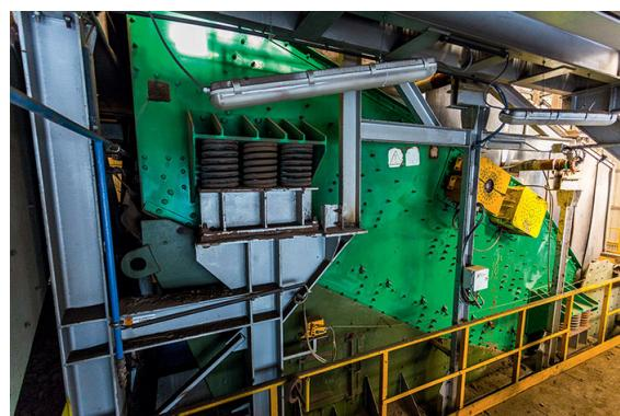
**Figure 2.** Vibrating screen machine (source: <https://kghm.com/pl/w-pracy>).
