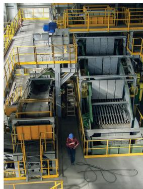
Figure 1. Vibrating screen machine (source: <https://kghm.com/pl/w-pracy>).
