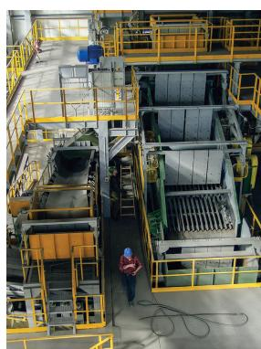
**Figure 1.** Vibrating screen machine (source: <https://kghm.com/pl/w-pracy>).
