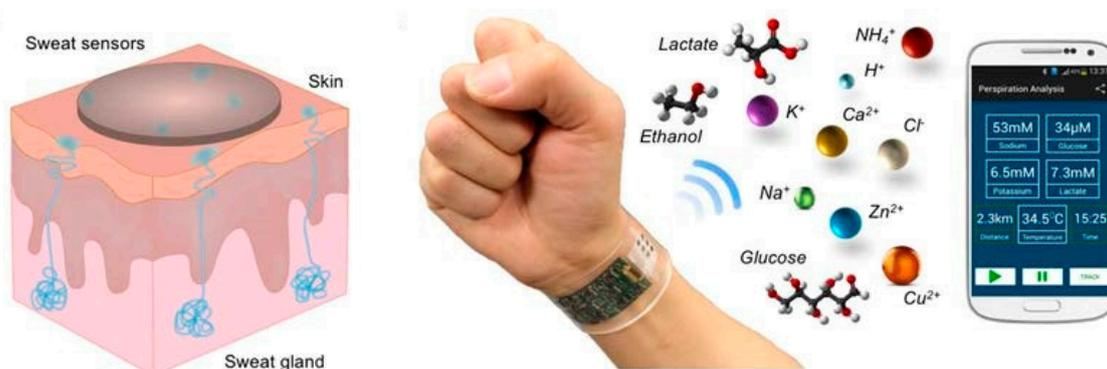
**Figure 7.** Wearable sweat biosensors which continuously measure a variety of sweat components for health monitoring. Reproduced from [164] with permission from IEEE.
