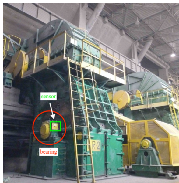
Figure 38. Hammer crusher with bearing and sensor locations marked.
