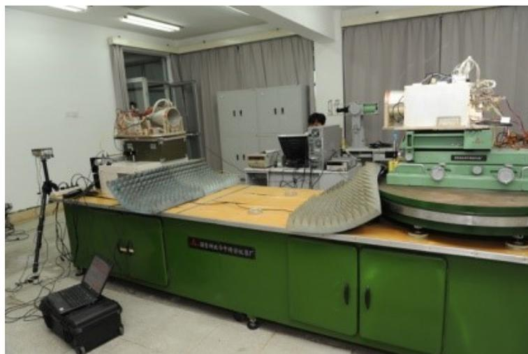
**Figure 7.** Six degree of freedom moving platform that achieved micron-level accuracy in position and an accuracy of milliarcseconds in attitude orientation.
