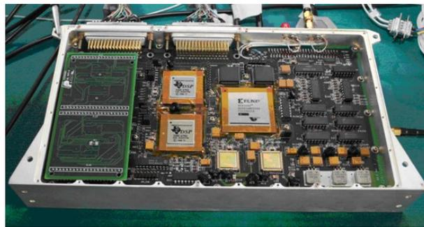
**Figure 4.** Signal processing hardware platform, including the K/Ka-band dual-frequency MWR processing module, BeiDou III B1C/B2a dual-frequency navigation processing module, and external interface module.
