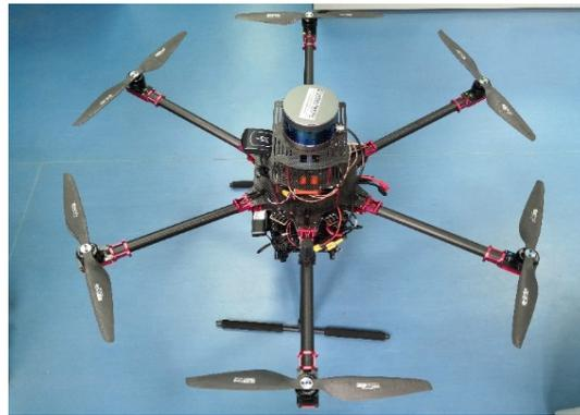
**Figure 6.** Our 8.5 kg drone platform (including paddles and batteries), which is equipped with three-dimensional (3D) Light Detection and Ranging (LiDAR), an RGB-D camera, an inertial measurement unit (IMU), an optical flow sensor (OFS), a barometer, and a global navigation satellite system (GNSS) receivers (BDS/GPS, RTK).
