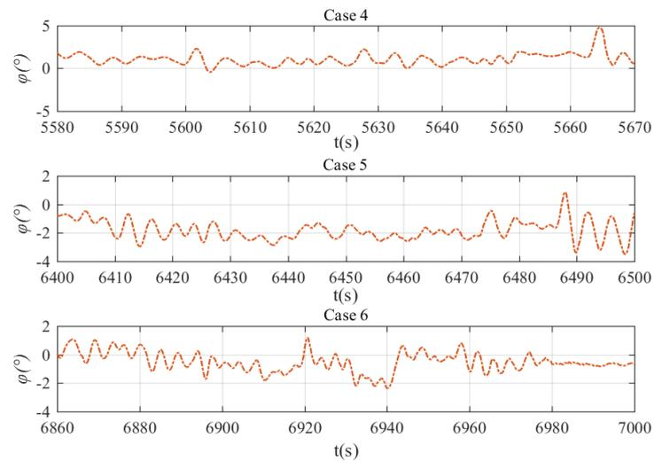
**Figure 24.** Roll angle during heading and depth control with rudder jam. Roll angle in case 4 (top), roll angle in case 5 (middle), and roll angle in case 6 (bottom).
