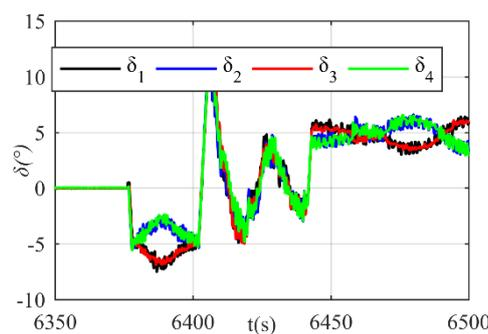
**Figure 18.** The actuator's control inputs derived from normal command transformation.
