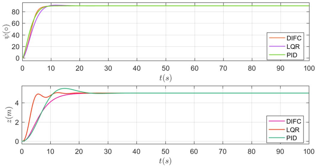
**Figure 11.** Simulation results when surge velocity is 3 kn. Realtime heading angle  $\psi$  during the first scenario (top), and the depth  $z$  of the vehicle (bottom).
