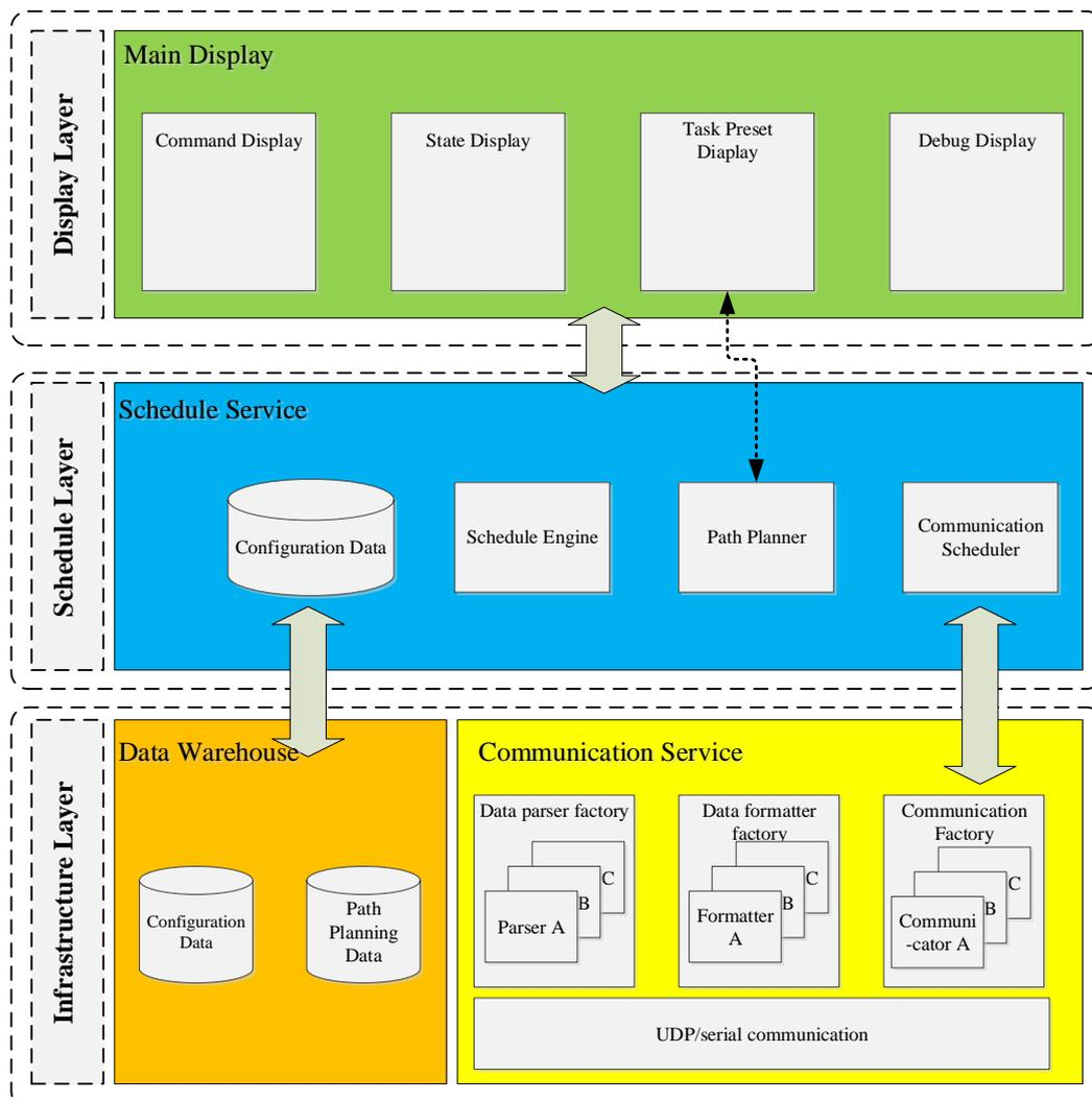
Figure 4. Architecture of factory method-based monitor software.
