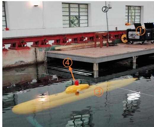
**Figure 1.** The xAUV sailing in the towing tank. (1) Portable surface monitor; (2) Surface WIFI antenna; (3) xAUV; (4) Integrated WIFI&GPS antenna.
