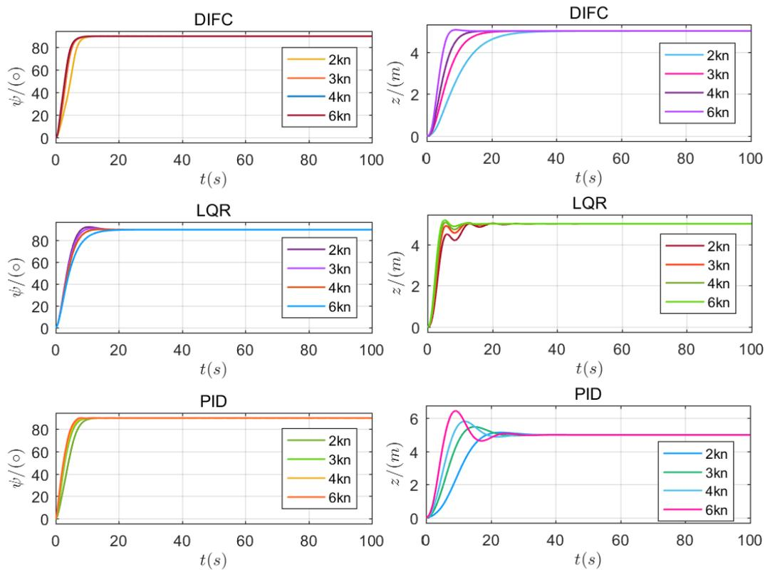
**Figure 12.** Simulation results under all predefined surge velocity (2 kn, 3 kn, 4 kn, 6 kn). Figures in the first line show the results of DIFC, the second line for LQR, and the third line for PID.
