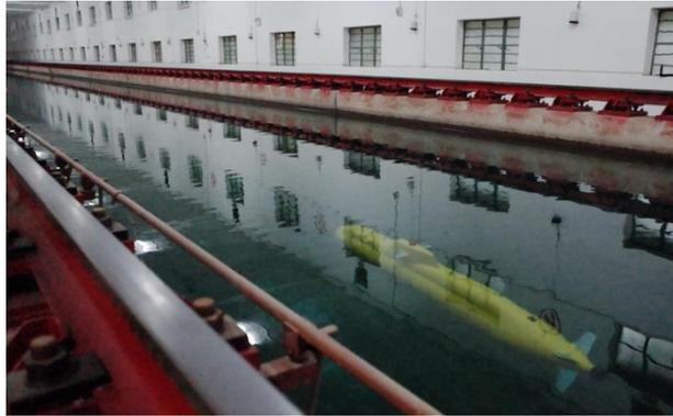
**Figure 13.** The xAUV is sailing in the towing tank.
