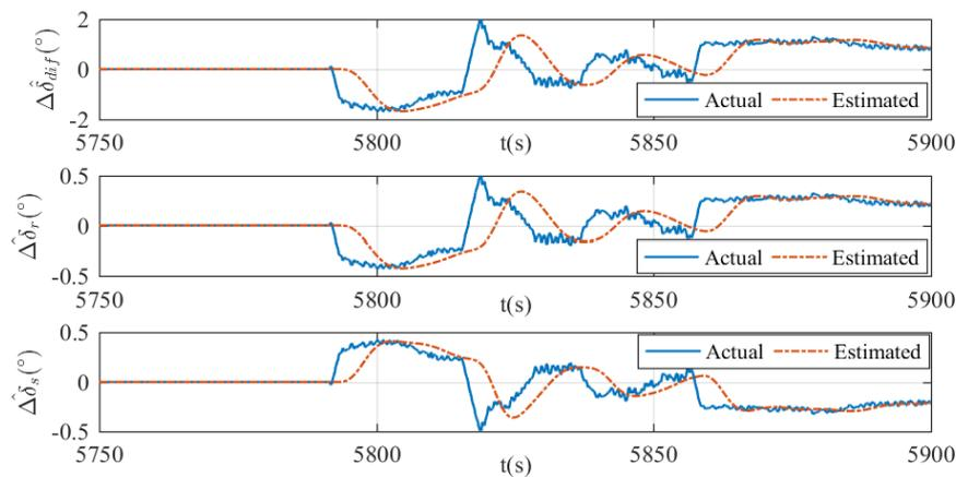
**Figure 21.** Estimation of  $\Delta u$  in case 3. The estimated differential angle (top), the estimated virtual vertical rudder angle (middle), and the estimated virtual horizontal rudder angle (bottom).
