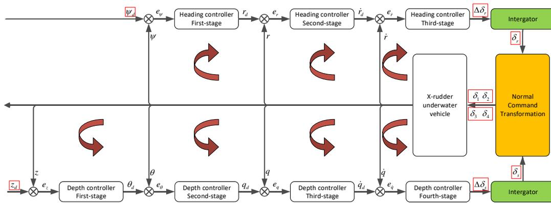
**Figure 8.** Principle diagram of DIFC.  $\delta_r$  and  $\delta_s$  are virtual vertical and horizontal rudder commands respectively.  $\Delta\delta$  is the increment,  $\delta_i (i = 1, 2, 3, 4)$  is the actuator's control input.  $e_s$  represents the error.  $\psi$  is the heading angle,  $r$  is the yaw rate,  $\dot{r}$  is the yaw acceleration,  $z$  is the depth,  $\theta$  is the pitch angle,  $q$  is the pitch rate, and  $\dot{q}$  is the pitch acceleration.
