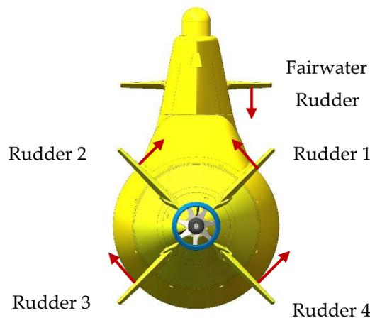
Figure 7. Sign definition of deflection angle. The red arrow represents the positive deflection.
