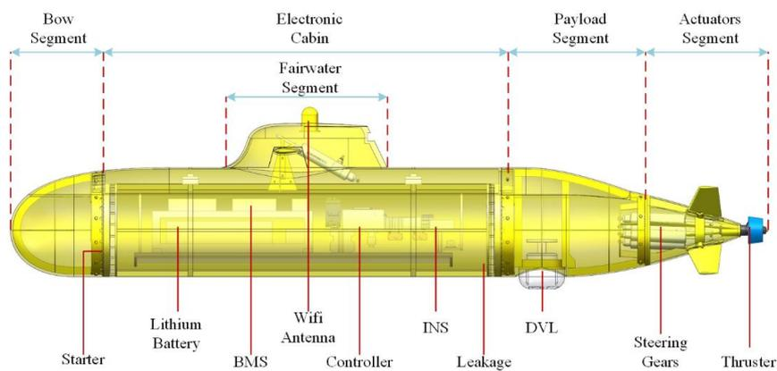
**Figure 2.** Layout of the xAUV.
