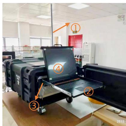
**Figure 3.** Surface monitor, including (1) WIFI antenna; (2) KVM; (3) Computer; (4) Display interface.
