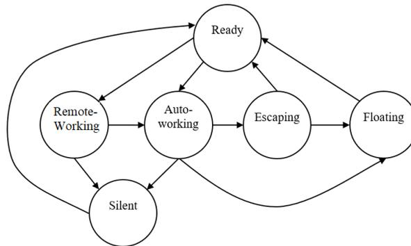
Figure 6. State transition diagram of FSM adopted by onboard software.
