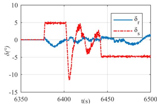
**Figure 17.** Virtual rudder commands from DIFC. The first stage (6375–6400 s), The second stage (6400–6445 s), The third stage (6445–6500 s).
