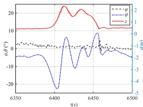
**Figure 14.** Depth control results. The red line is the depth, the blue line is the pitch angle, and the black line is the roll angle.
