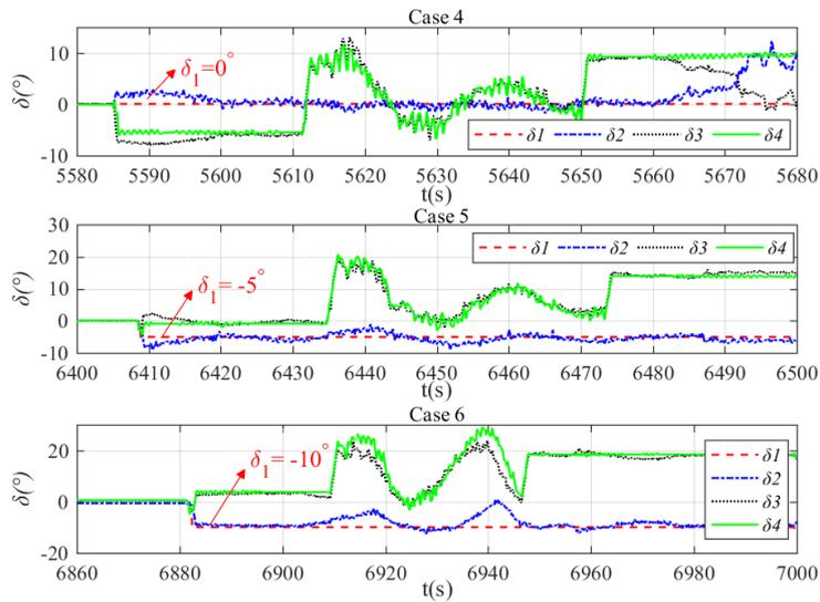
**Figure 23.** Results of NLP-based command transformation with rudder jam. Rudder commands in case 4 (top), rudder commands in case 5 (middle), and rudder commands in case 6 (bottom).
