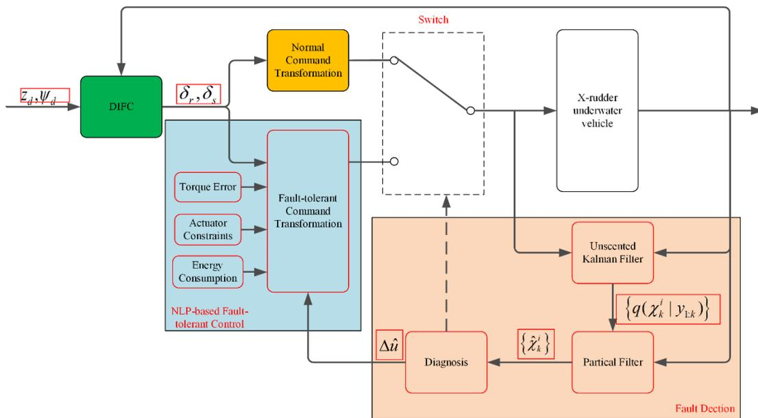
Figure 10. Control block diagram of fault-tolerant steering prototype.
