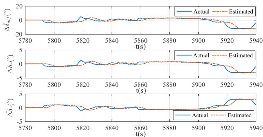
**Figure 20.** Estimation of  $\Delta u$  in case 2. The estimated differential angle (top), the estimated virtual vertical rudder angle (middle), and the estimated virtual horizontal rudder angle (bottom).
