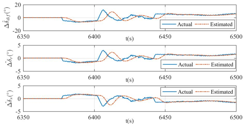
**Figure 19.** Estimation of  $\Delta u$  in case 1. The estimated differential angle (top), the estimated virtual vertical rudder angle (middle), and the estimated virtual horizontal rudder angle (bottom).
