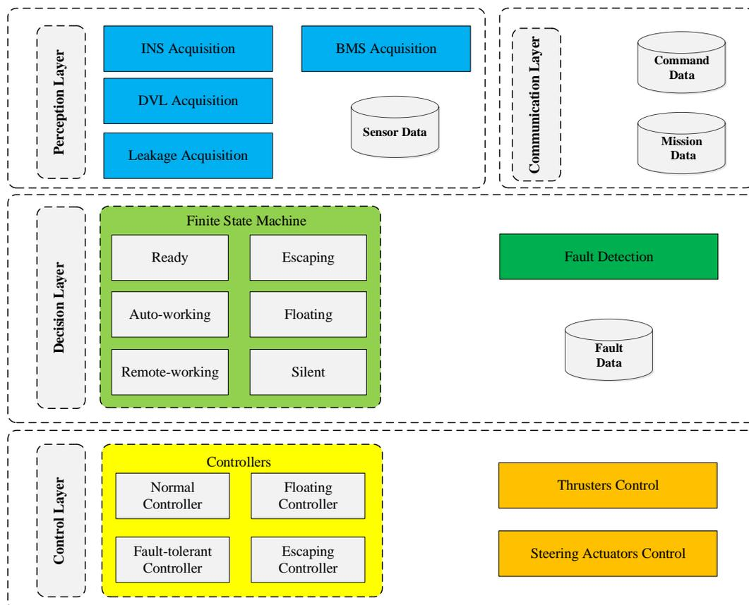
Figure 5. Architecture of FSM-based onboard software.
