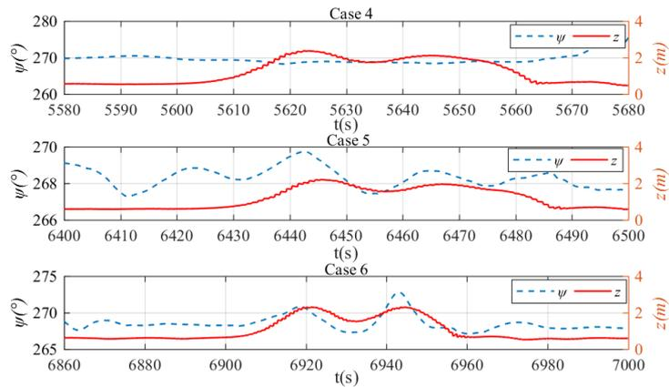
**Figure 22.** Results of depth and heading control with rudder jam. Heading and depth in case 4 (top), heading and depth in case 5 (middle), and heading and depth in case 6 (bottom).
