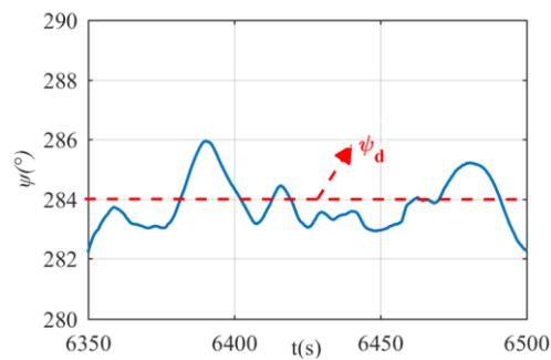
**Figure 15.** Heading control results. The blue line is the heading angle and the red line is the desired heading.
