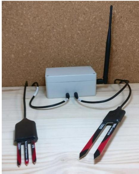
**Figure 4.** Node with ECH2O soil moisture sensors.
