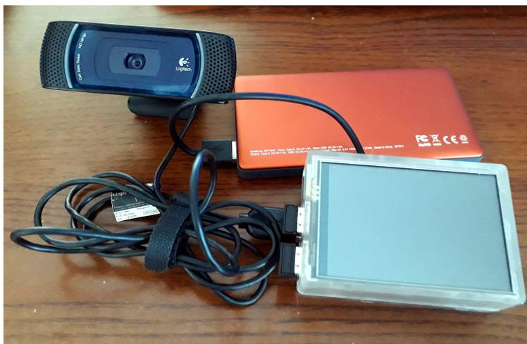
**Figure 4.** The assembled microcomputer that was used in this research. It consists of a Raspberry Pi 3 model B+ in a semi-transparent case with a 3.5" LCD touchscreen, a Logitech Webcam C920 HD Pro, and a powerbank (5 V, 3 A).
