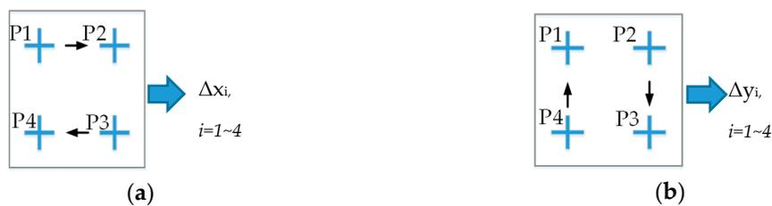
**Figure 2.** Motion of the cross-hair marks in the calibration process, in which, from P1 to P4, are reference points;  $\Delta x_i, \Delta y_i$ : are pixel distances between the two adjacent points along the  $x$  axis and the  $y$  axis, respectively. (a,b) show the travel of the cross-hair mark along  $x$  and  $y$  axis directions, respectively.
