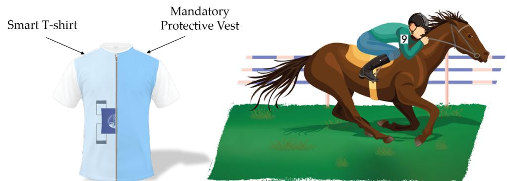
**Figure 5.** Schematic representation of how the wearable system is worn during the race (underneath the protective vest).
