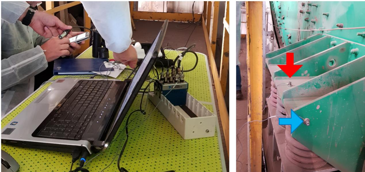
**Figure 3.** Computer and data acquisition card used for the experiment (left image) and positioning of horizontal and vertical direction sensors on the bottom right spring set (right image).
