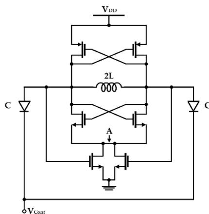
**Figure 2.** Schematic of a CMOS LC-VCO with the switched-biasing technique to the current source (reproduced with permission from the author, RF CMOS low-phase-noise LC oscillator through memory reduction tail transistor; published by IEEE, 2004) [34].
