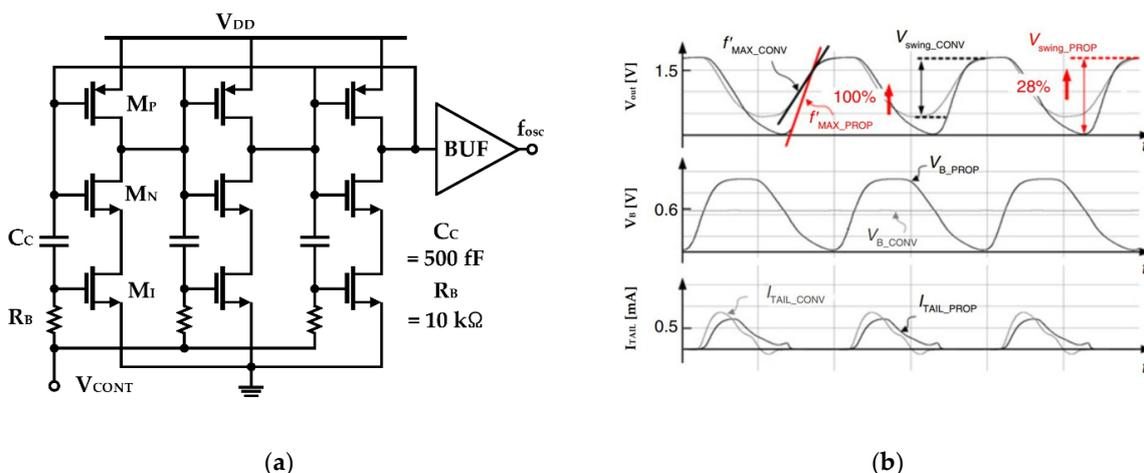
**Figure 12.** Ring VCO using the switched-biasing technique: (a) schematic; (b) simulated waveforms of the VCO output (top), bias voltage of the current source (middle), and tail current of the inverter cell (bottom) (reproduced with permission from the author, Low phase noise ring VCO employing input-coupled dynamic current source; published by IET, 2020) [61].
