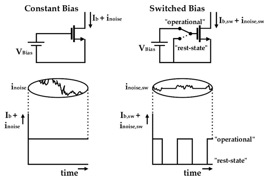
**Figure 1.** Conceptual diagram of switched-biasing technique (reproduced with permission from the author, reducing MOSFET  $1/f$  noise and power consumption by switched biasing; published by IEEE, 2000) [33].
