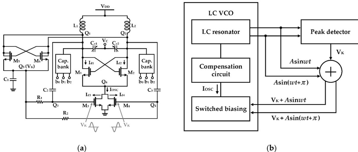
**Figure 13.** VCO using self-biasing with the adaptive DC voltage: (a) schematic; (b) operation of the self-biasing with the adaptive DC voltage from peak tracking at the oscillator outputs (reproduced with permission from the author, Low voltage CMOS LC VCO with switched self-biasing; published by Wiley, 2009) [63].
