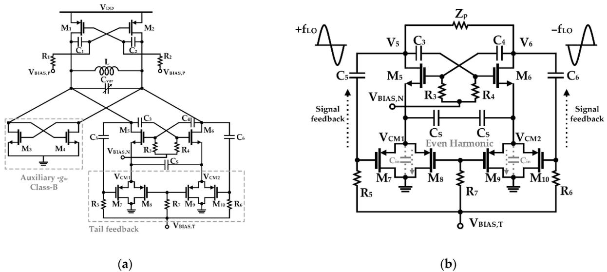
**Figure 11.** Class-C CMOS VCO using the switched-biasing technique: (a) schematic of the VCO; (b) bias conduction at the sub-threshold operation of the split current sources implemented by PMOS transistors (reproduced with permission from the author, A 2.2 to 2.9 GHz complementary class-C VCO with PMOS tail-current-source feedback achieving  $-120$  dBc/Hz phase noise at 1 MHz offset; published by IEEE, 2019) [54].
