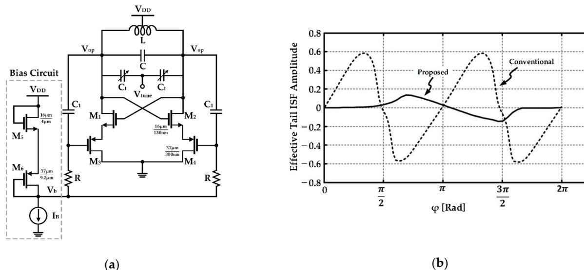
**Figure 10.** CMOS VCO based on the ISF manipulation technique: (a) schematic of the VCO including current sources using PMOS transistors; (b) waveforms of the effective tail ISF amplitude for the conventional current source using NMOS and the proposed current source using PMOS (reproduced with permission from the author, a 2.4 GHz VCO with FOM of 190dBc/Hz at 10 kHz-to-2 MHz offset frequencies in 0.13  $\mu\text{m}$  CMOS using an ISF manipulation technique; published by IEEE, 2015) [60].
