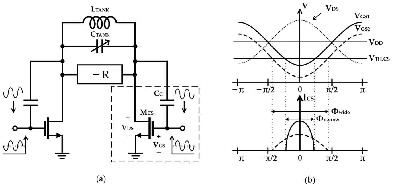
**Figure 17.** Conduction angle in the VCO operation: (a) description of the conduction angle in the VCO; (b) comparison of the conduction angle between the constant-biasing and the switched-biasing techniques.
