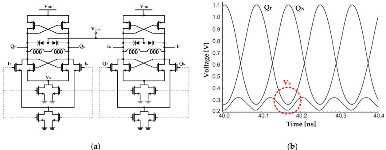
**Figure 5.** CMOS quadrature-VCO (QVCO) with separate current sources based on the switched-biasing technique: (a) schematic of the QVCO; (b) simulation waveforms at the outputs of the quadrature channel and the common node (reproduced with permission from the author, Low-phase-noise CMOS quadrature VCO; published by IEEE, 2006) [57].
