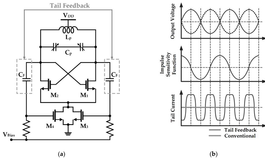
**Figure 6.** Millimeter-wave NMOS VCO using the switched-biasing technique: (a) schematic of the VCO; (b) waveform analysis of the VCO based on the ISF theory (reproduced with permission from the author, a low phase noise quadrature injection locked frequency synthesizer for mm-wave applications; published by IEEE, 2011) [51].
