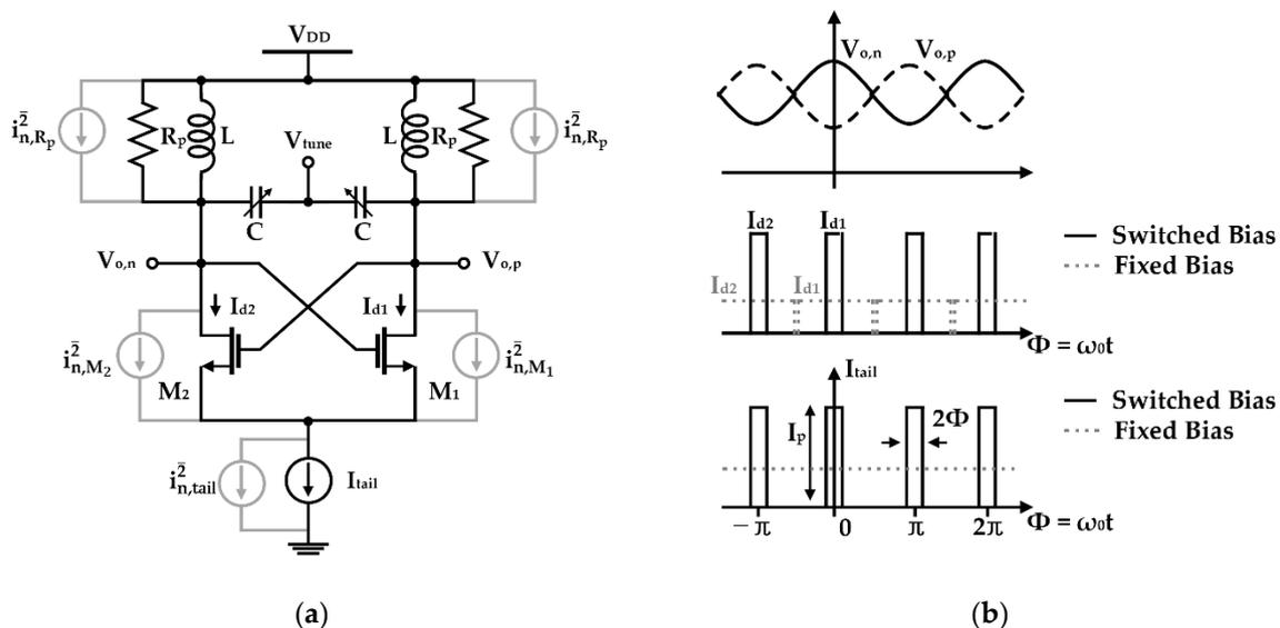
**Figure 3.** Analysis of VCO characteristics depending on the pulse modulation of the current source using the impulse sensitivity function theory: (a) schematic of the differential LC-VCO; (b) conceptual waveforms of the output voltages and drain currents of the VCO and the bias current by the pulse-modulated current source (reproduced with permission from the author, Tail current-shaping to improve phase noise in LC voltage-controlled oscillators; published by IEEE, 2006) [47].
