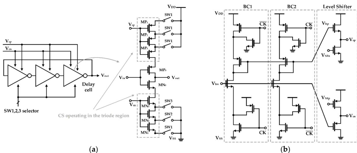
**Figure 4.** Ring VCO based on a switched-bias circuit (SBC): (a) block diagram of the ring VCO and schematic of the delay cell in the VCO; (b) schematic of SBC for current source modulation (reproduced with permission from the author, Low-voltage, low-phase-noise ring voltage-controlled oscillator using  $1/f$ -noise reduction techniques; published by The Japan Society of Applied Physics, 2007) [50].
