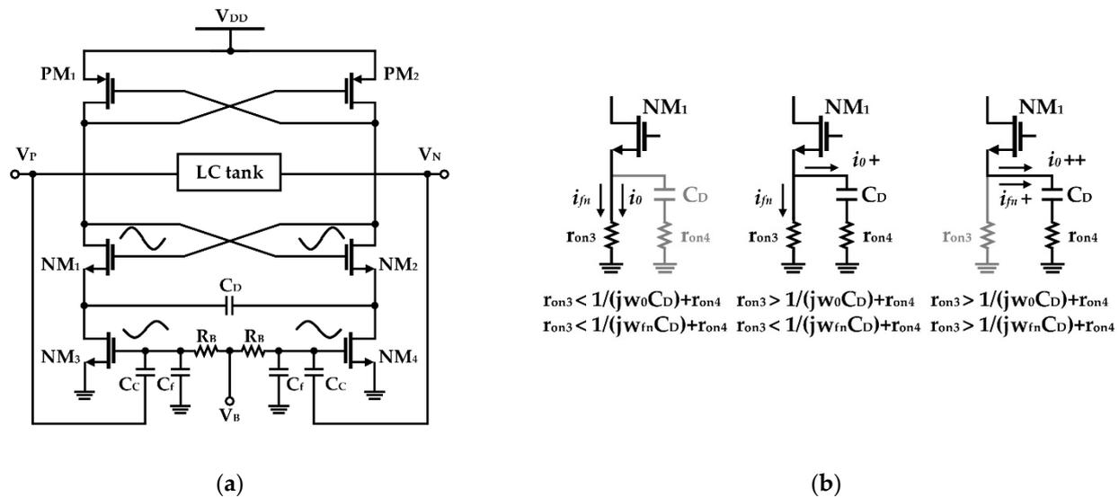
**Figure 8.** CMOS VCO including degeneration and filter capacitors: (a) schematic of the VCO; (b) current flows depending on the capacitance of  $C_D$ —the usage of the optimal capacitance can divide the current into two paths, as shown in the middle case (reproduced with permission from the author, Reduction of  $1/f^3$  phase noise in LC oscillator with improved self-switched biasing; published by Springer, 2015) [58].
