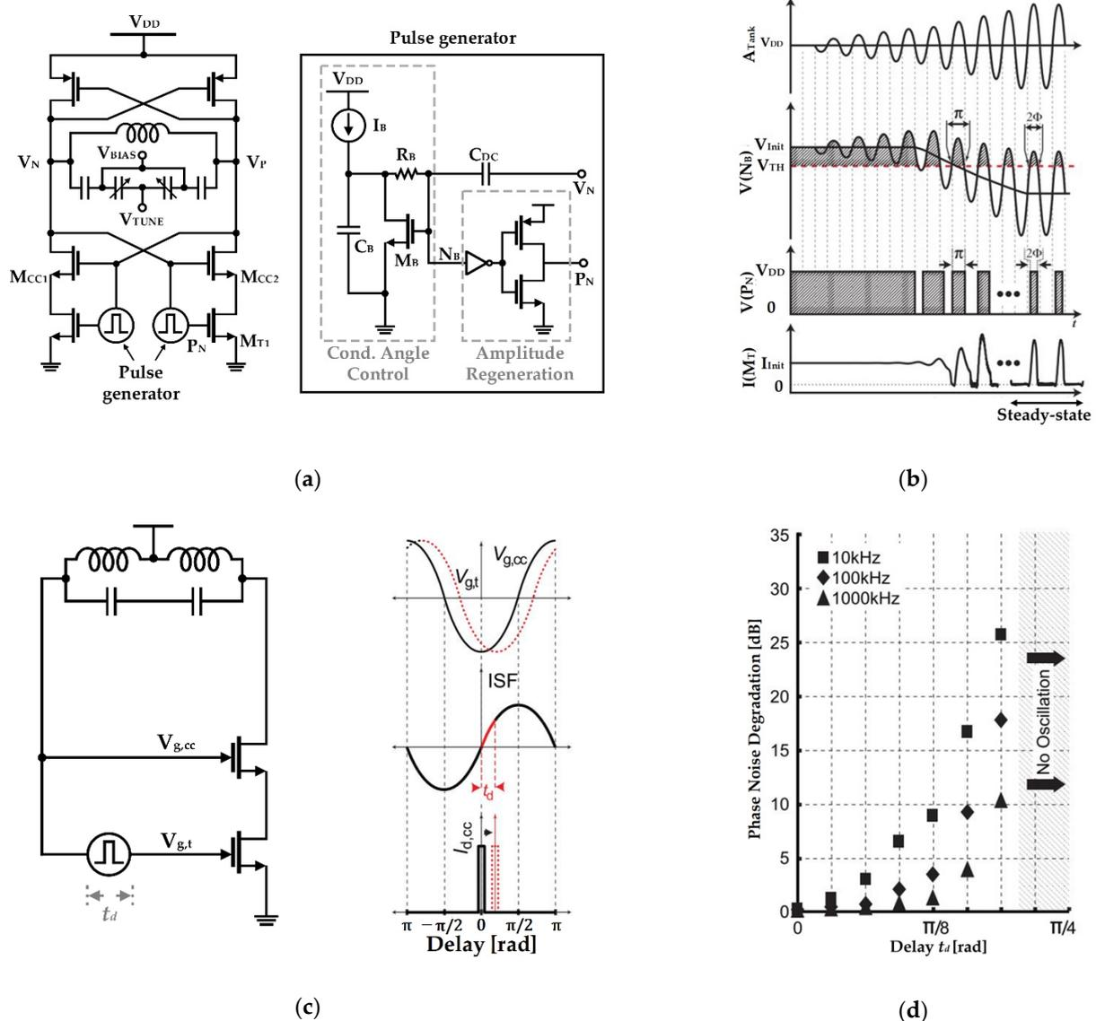
**Figure 14.** VCO employing the pulse generator that supplies pulse waveforms and the adaptive DC bias voltage: (a) schematic; (b) conceptual diagram of the VCO including the pulse generator operation; (c) intrinsic delay of the pulse generator; (d) simulated phase noise degradation with increasing the delay of the pulse generator (reproduced with permission from the author, A pulse-tail-feedback LC-VCO with 700 Hz flicker noise corner and  $-195\text{dBc}$  FoM; published by IEICE, 2019) [64].
