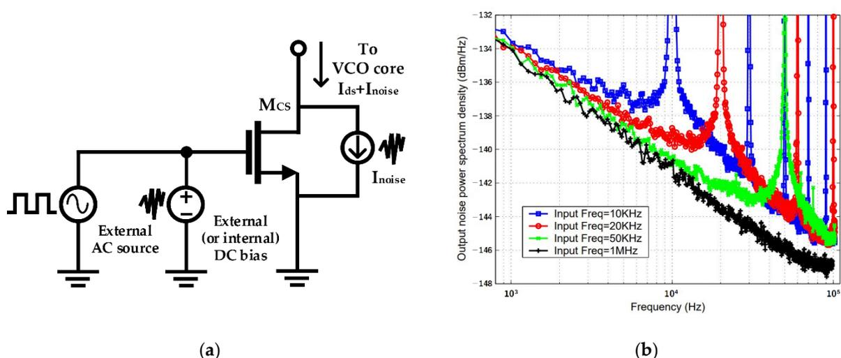
**Figure 15.** Characteristic of external-biasing topology: (a) conceptual schematic of external biasing (also available in PMOS configuration); (b) large noise peaks appearing as harmonics of the modulation frequency correlated with the external signal (reproduced with permission from the author, Experimental study on MOSFET's flicker noise under switching conditions and modelling in RF applications; published by IEEE, 2001) [56].
