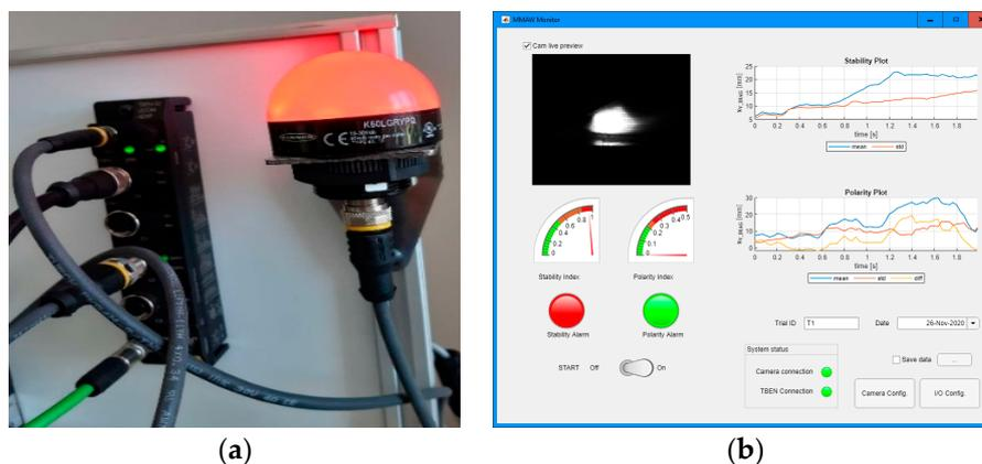
**Figure 22.** (a) View of I/O module—Turck TBEN TBEN-S2-2COM-4DXP, Turck GmbH & Co. KG, Mulheim, Germany, and indicating light Banner K50LGRYPQ; (b) screenshot of System A GUI, made in Matlab App Designer.
