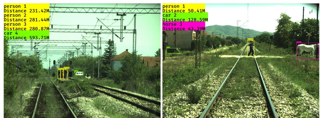
**Figure 6.** DisNet estimation of distances to objects in a rail track scene from the RGB camera image (extracted from [61]).
