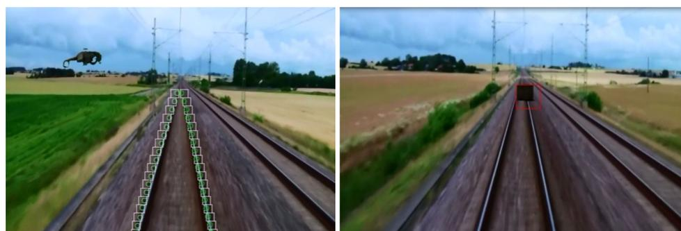
**Figure 2.** Detection of objects in the ROI—region of detected rail tracks. **(left)** Windows-based systematic search for objects along the detected rail tracks ([17,41]); **(right)** digitally added stationary object and its detection ([17,41]).
