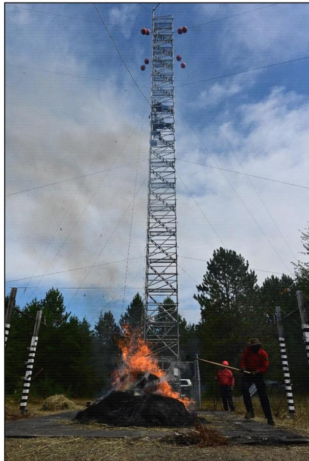
**Figure 3.** Example of experimental burn trials conducted 18 September 2019 during this experiment. Pictured here, researchers add fuel to a ~2 m diameter fire with a pitchfork while it is sampled by Bomberos and the reference FLIR imager on the tower adjacent to the burn platform.
