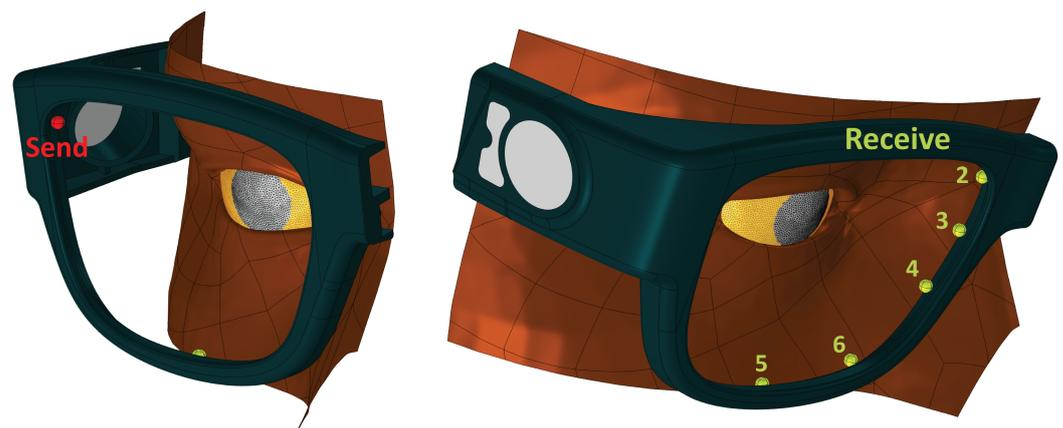
**Figure 1.** Physical layout for our model. Send location: transducer operating in transmit mode; numbered locations: transducers operating in receive mode. The distance traveled by a ray starting at the send position, reflecting off the cornea, and arriving at receiver 4 is in the 5.28 to 5.35 mm depending on gaze.
