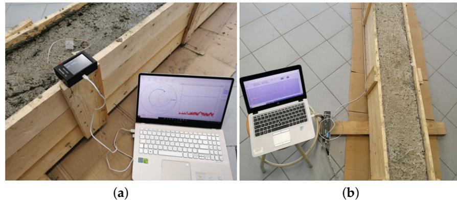
**Figure 3.** Experimental setup for measurements on the concrete beam: (a) nanoVNA with PCP for FDR measurements; (b) TDR with d-SE for TDR measurements.
