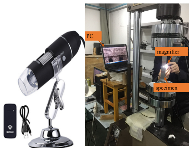
Figure 10. Experiments for collecting crack data: the left image shows the measuring magnifier used in the experiments, and the right image shows the experimental environment.
