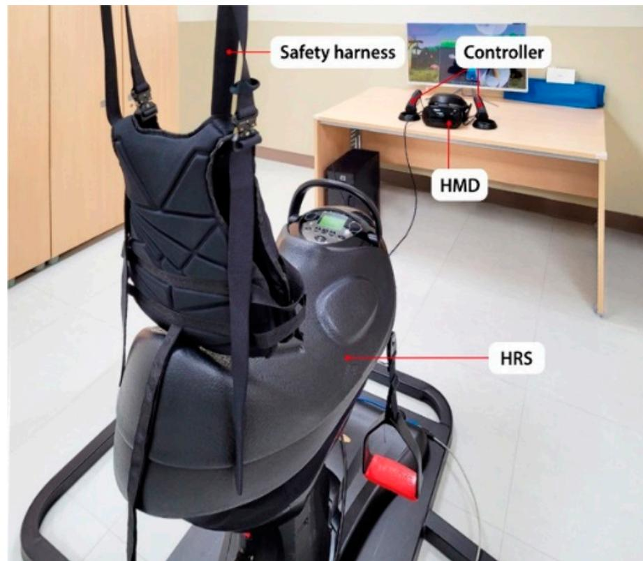
**Figure 1.** Architecture of the proposed virtual reality (VR)-incorporated horse riding simulator (HRS).
