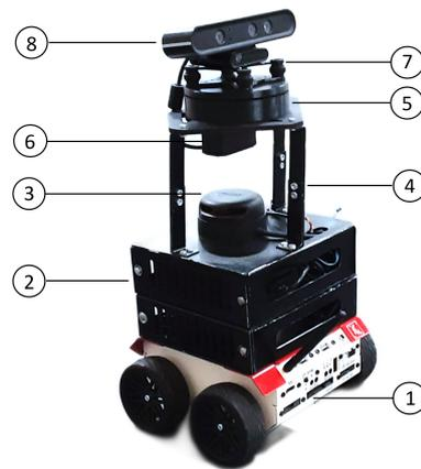
**Figure 2.** An overview of the mechanical design of ROBOGait. The figure shows: (1) the mobile robotic base, (2) on-board computer (Intel NUC), (3) Slamtec LIDAR A2 sensor, (4) adjustable aluminum brackets, (5) servoing system mechanism, (6) servomotor (Hitec HS-755HB), (7) damping device, and (8) Orbbec Astra RGBD camera.
