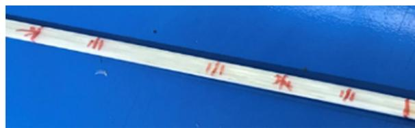
**Figure 5.** Sensorized FRP beam test piece.
