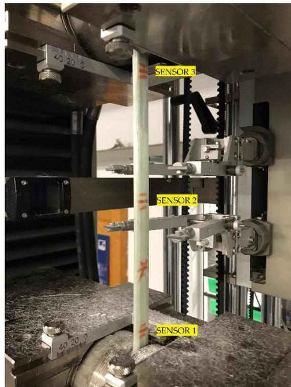
Figure 6. Sensorized beam test piece setting.
