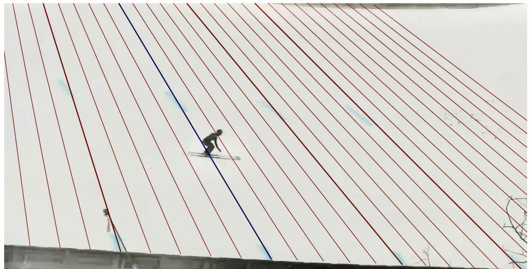
**Figure 3.** Example for the manual determination of the official video-based jumping distance. The red lines are the calibrated projection of the official jumping distance (to the jump-off platform). The blue line corresponds to the determined jumping distance.
