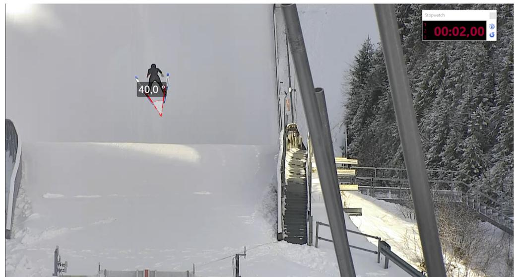
**Figure 5.** Example of the manual labeling of the V-angle 2 s after the crossing of the jump-off platform. The PTZ camera is mounted at the top of the in-run.
