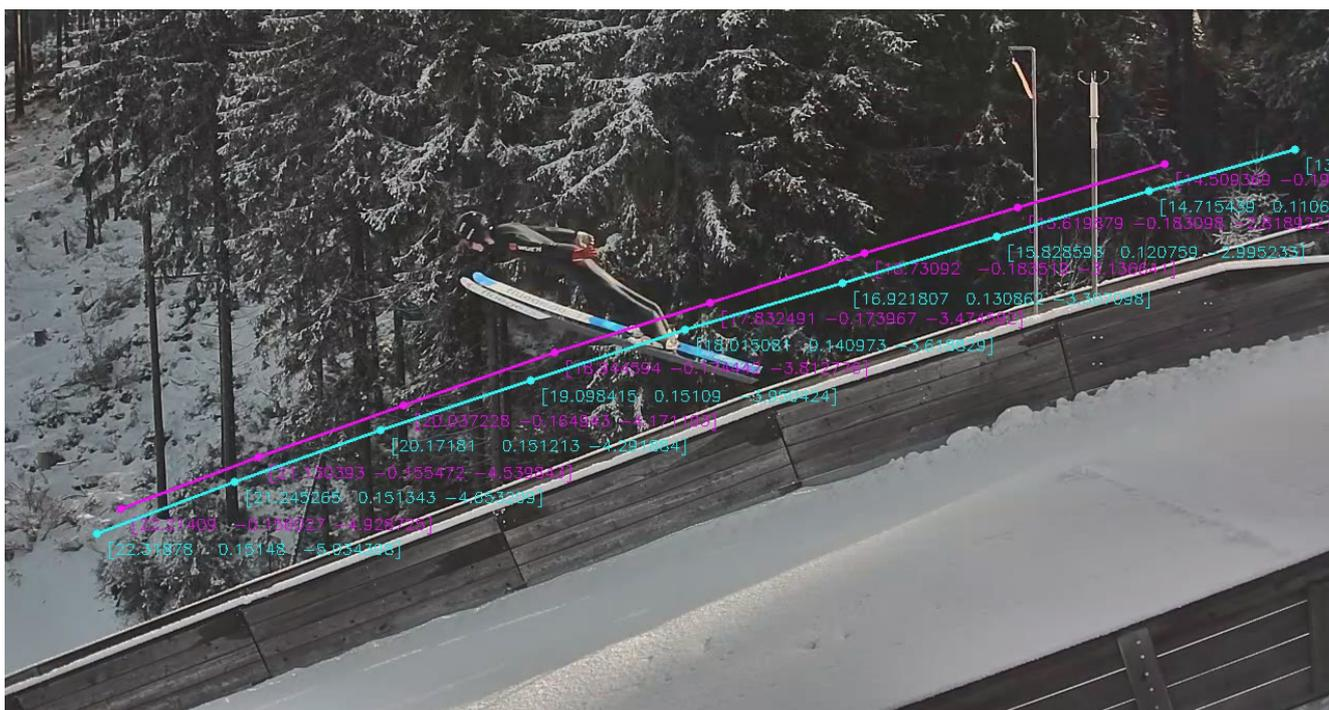
**Figure 7.** Projection of the WRTTS position data onto the video of the camera at 18 m after take-off. The cyan curve shows the trajectory of the WRTTS tracker placed on the binding of the left foot. The magenta curve shows the trajectory of the right tracker. The numbers indicate the corresponding 3D coordinates in meters. Coordinates as depicted in Figure 1.
