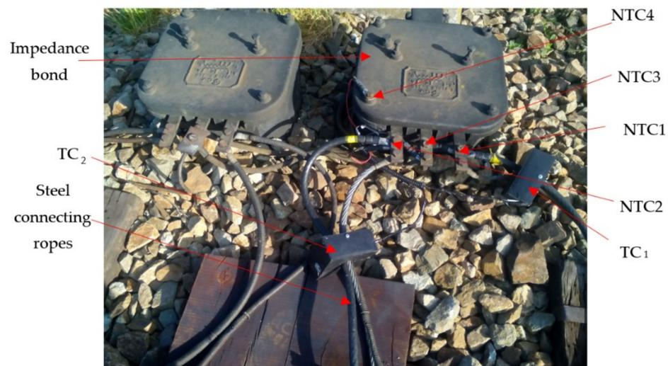
**Figure 10.** Image of the current and temperature transducers mounted in return circuit of oil impedance bond in the field.
