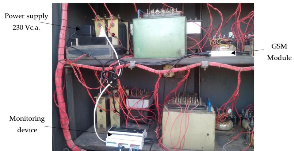
**Figure 11.** Image of the monitoring device in the relay cabinet from the field.
