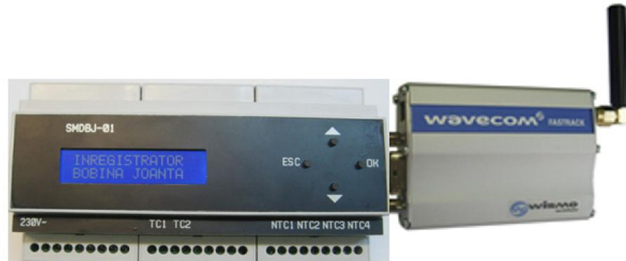
**Figure 7.** Monitoring device of return circuit using GSM communication.
