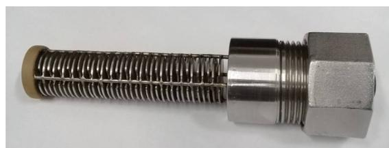
Figure 9. Proposed capacitive sensor for determination of water content.
