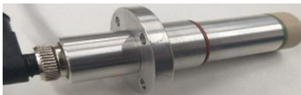
**Figure 10.** Proposed ultrasonic sensor for determination of density and flow.
