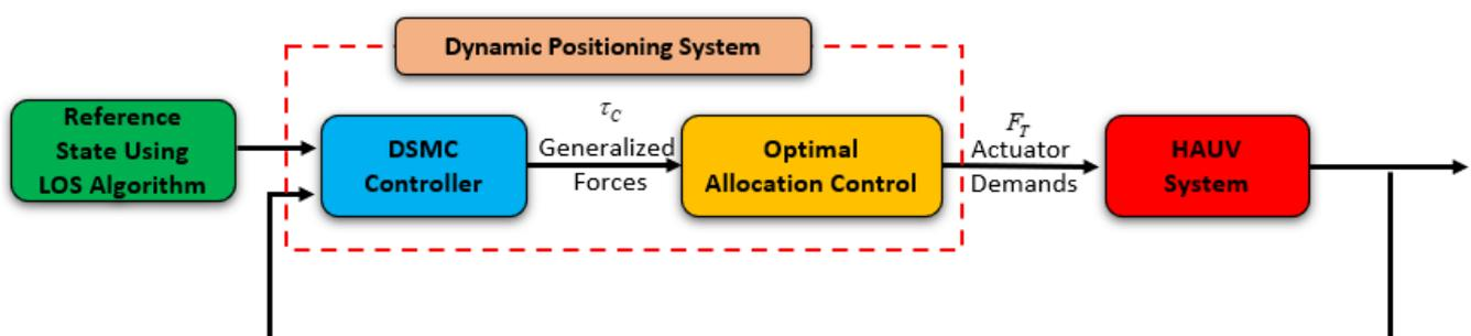
Figure 4. A dynamic positioning (DP) control system, including a motion control law and an allocation control module.
