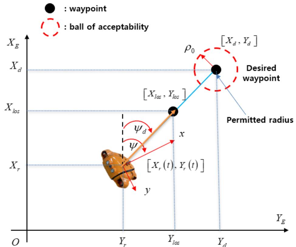
Figure 3. The proposed line of sight (LOS) method and the target waypoint.
