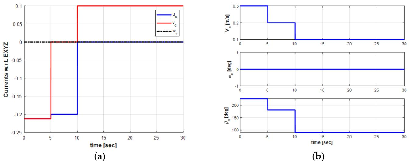
**Figure 6.** Ocean current form: (a) ocean current vector w.r.t Earth–fixed coordinate; (b) ocean current parameters.
