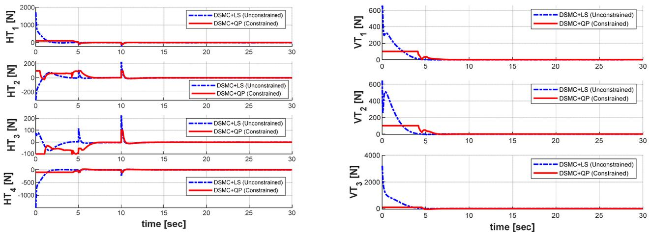
Figure 15. Seven thruster forces in both cases: (a) four horizontal thrusters; (b) three vertical thrusters.
