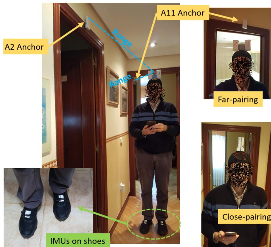
**Figure 17.** Apartment details, showing some examples of anchors locations, tags mounted on a cap on the actor's head in both pairing configurations, and IMUs attached on shoes.
