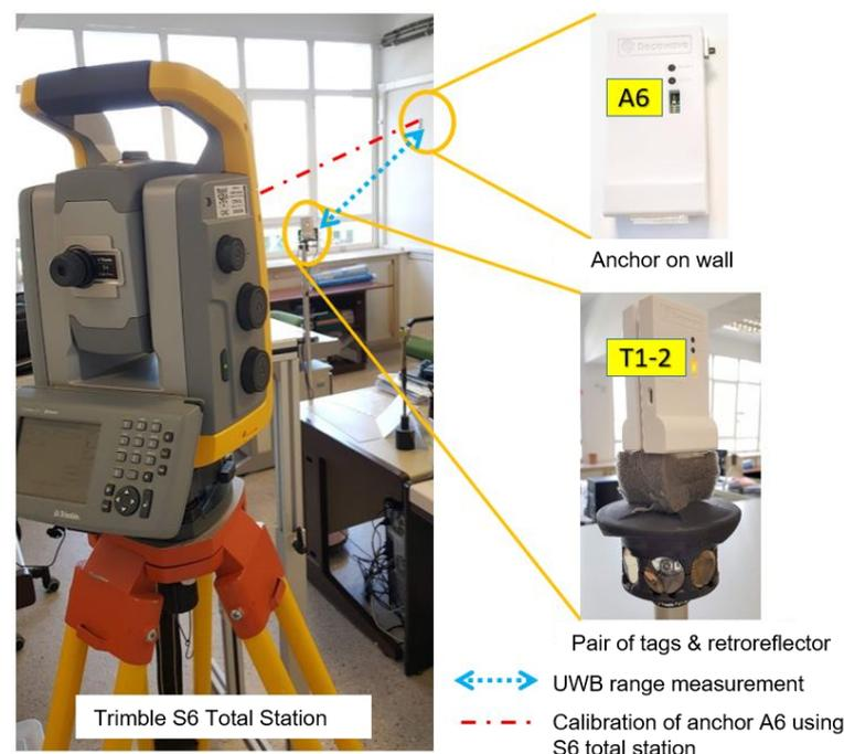
**Figure 11.** Experimental environment with the precision equipment (Trimble S6 Total Station) to calibrate the position of anchors and to track the tags obtaining the true position or GT (Ground-Truth).
