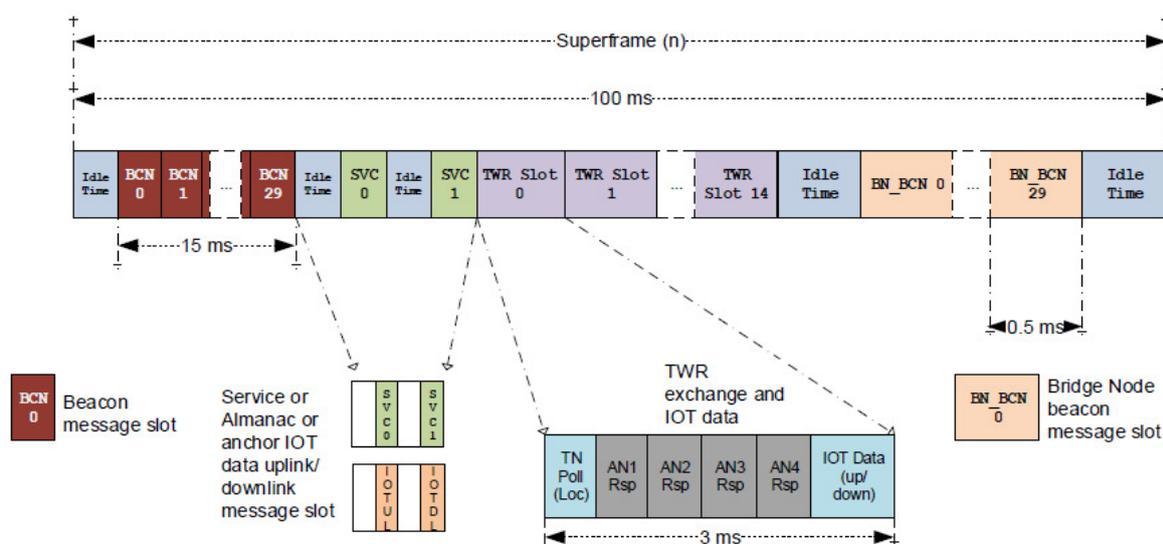
**Figure 3.** Superframe of Decawave’s PANS protocol for its DWM1001 modules. The protocol limits to four anchors the maximum number of ranges that each tag can measure within its TWR slot. However, it is quite scalable in the number of tags which can be operative at the same time—for example, 15 tags every 100 ms, or 150 tags at 1 Hz [22].
