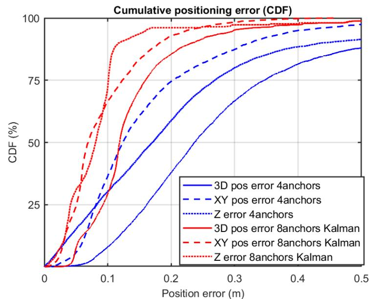
**Figure 15.** Location error in CDF (Cumulative Distribution Function), in the case of using four ranges (algorithm integrated in the tags by the manufacturer Decawave), and in the case of using eight ranges with an external algorithm based on the Kalman filter.
