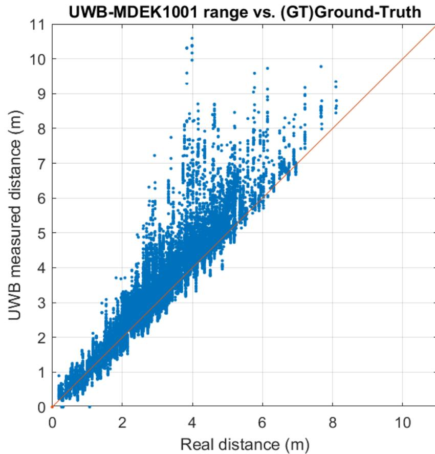
Figure 19. Real-distance vs. UWB measured distance (tag to anchors) at the apartment scenario.
