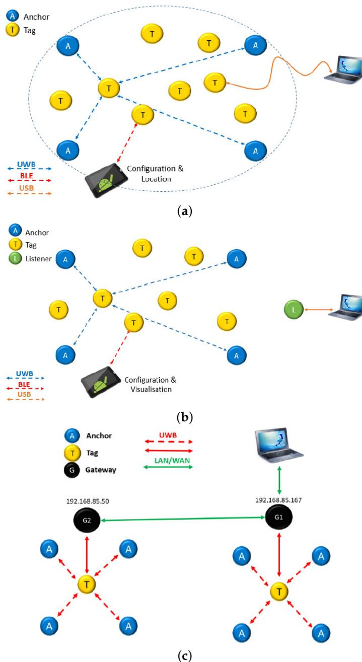
**Figure 2.** Different configurations of the DWM1001DEV modules to create a location network, and ways of monitoring: (a) normal mode with connection to individual tags (access to position of that tag and four ranges); (b) extended mode with listener to access positions of all tags in the network (not ranges); (c) extended mode with gateways to increase scalability of the deployment and also get access to positions of all the tags in the network (not ranges) [22].
