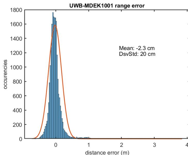
**Figure 13.** Errors in the measurement of ranges between eight anchors and four tags moving within our indoor lab space. Above: Measured vs. actual range. Below: error distribution, and overlapping Gaussian.
