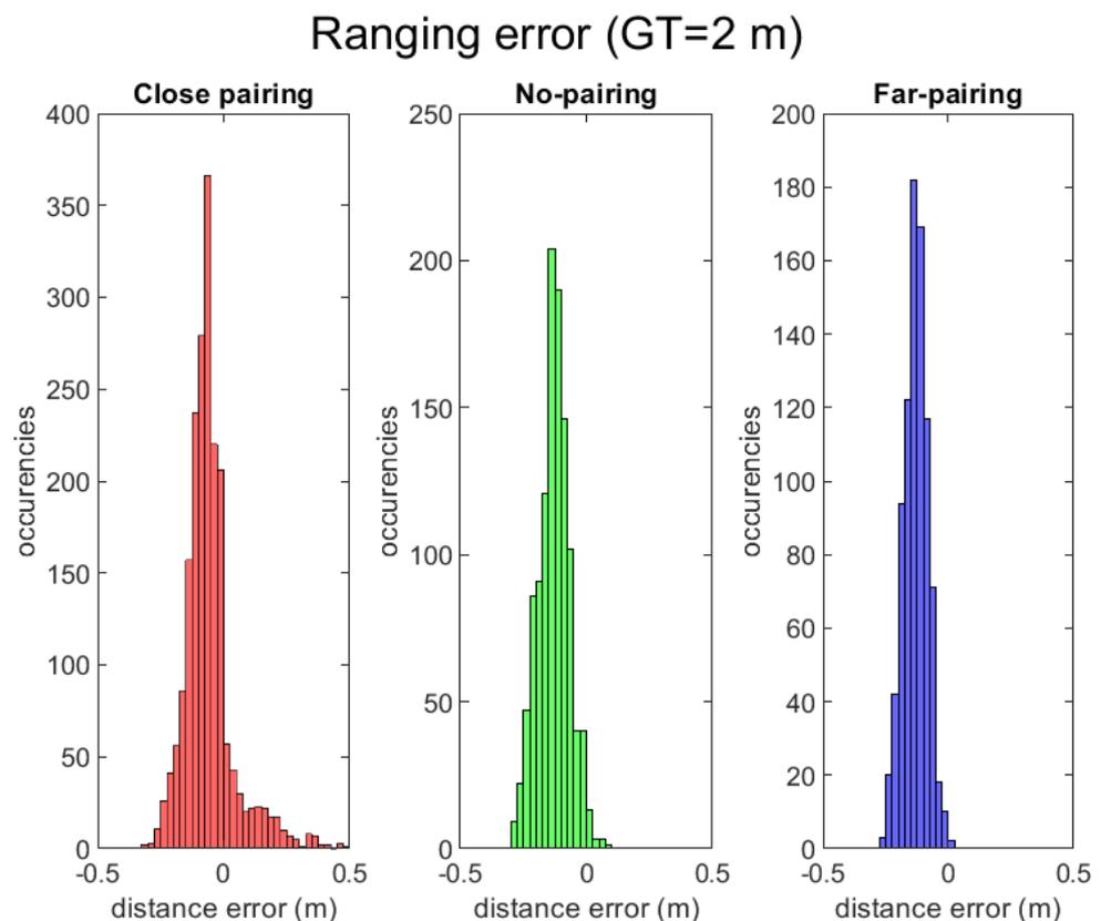
**Figure 8.** Ranging measurements at 2 m distance from a fixed anchor in LOS conditions. Effect of pairing tags in range errors for: Close pairing (red), No-pairing (green) and Far-pairing (blue).
