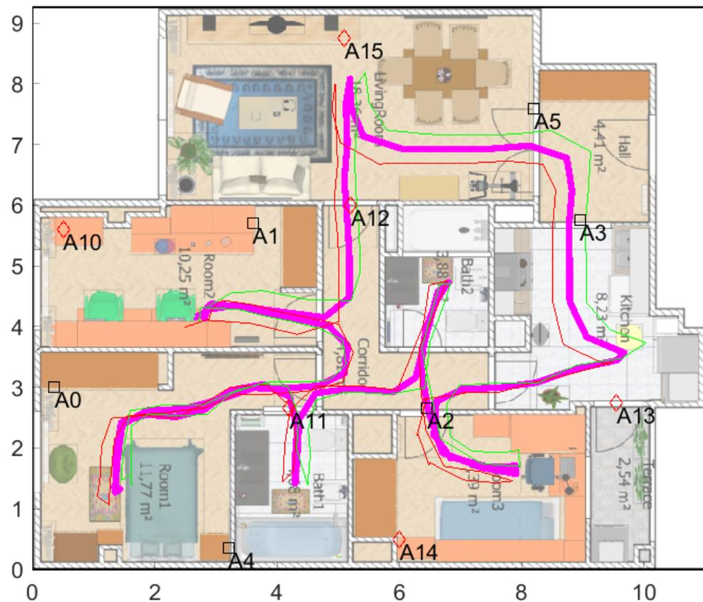
**Figure 16.** Apartment's floormap. A total of 12 anchors were deployed creating two networks of six anchors each (Net1: squares, and Net2: diamonds). A ground-truth for one of the experiments is marked with a magenta line.
