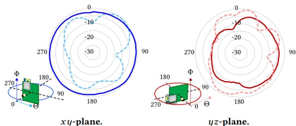
**Figure 6.** Radiation pattern of DWM1001 antennae in the horizontal ( $x$ - $y$ ) and vertical ( $y$ - $z$ ) planes with respect to the long axis of the tag’s enclosure [22,26].
