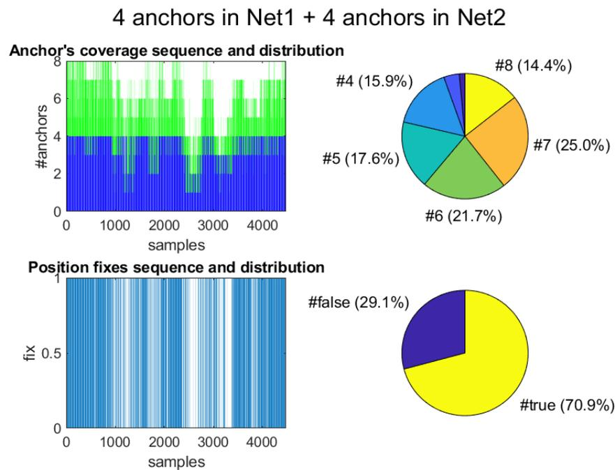
**Figure 18.** Coverage of anchors for one of the testing routes at the apartment. Top: Total number of anchors in view when considering the contribution of both tags in a pair (tag1&tag2). Bottom: Position fixes computed by the Decawave algorithm based on four anchors at a time.
