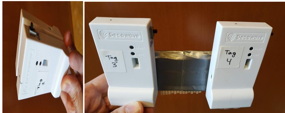
**Figure 7.** Pairing of tags: Close pairing (left) and Far-pairing (right).
