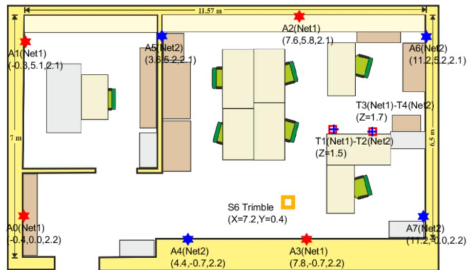
**Figure 10.** Test environment map-layout. The six-pointed stars indicate the eight anchors distributed in two interleaved sub-networks (Network1 in red, and Network2 in blue). T1-2 and T3-4 are two pairs of tags in static condition. The location of the Trimble S6 total station is marked in orange. The previous Figure 9 is a view of our lab from point A7 (bottom right corner).
