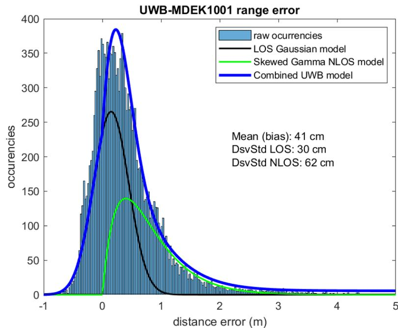
Figure 20. Error distribution in ranging (tags to anchors) at the apartment scenario An NLOS model (blue) is overlaid on the experimental histogram.
