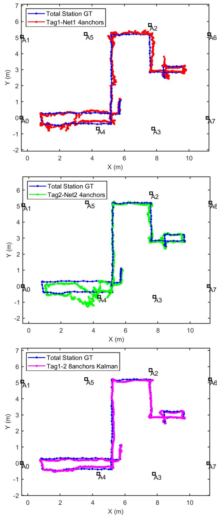
**Figure 14.** Location results with the estimation methods proposed in this work, and comparison with the ground-truth (GT) supplied by the S6 Total station. Top: Tag1 estimation by Decawave algorithm with four ranges in Network1. Middle: Tag2 estimation by the Decawave algorithm with four ranges in Network2. Bottom: Tag1-Tag2 pair estimation by EKF algorithm with eight ranges using both networks.
