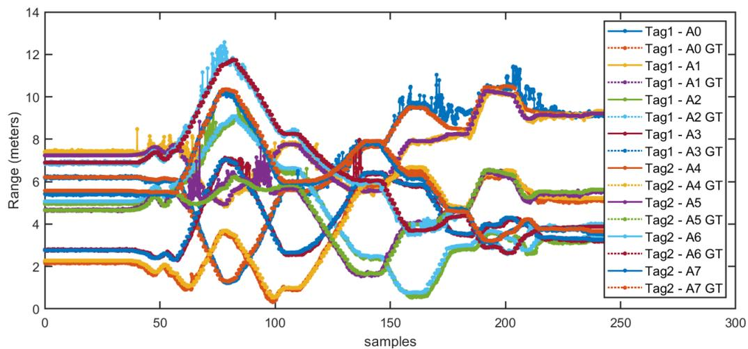
**Figure 12.** Range estimations between different anchor to tag vs. the GT (ground-truth) range.
