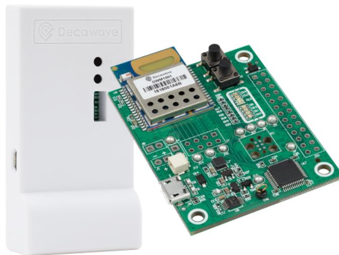
**Figure 1.** Configurable UWB module (DWM1001DEV) in the MDEK1001 evaluation kit from Decawave (the kit contains 12 such modules); left: housing; right: DWM1001 circuit board with the antenna on top [22].
