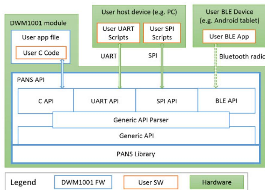
**Figure 4.** The four types of API through which we can individually access the ranges of each tag. There is an embedded API in the DWM1001 module accessible in C language, and other APIs to access by means of external equipment to the DWM1001 module through wired (serial COM) or wireless (BLE) connections [22].
