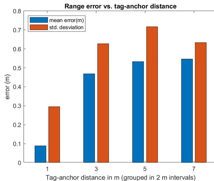
**Figure 21.** Mean and standard deviation of the measured range error in four groups of range bins: 0–2 m, 2–4 m, 4–6 m, and 6-Infinite. Information is obtained from the same data as in Figures 19 and 20.
