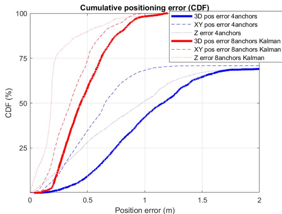
**Figure 23.** Cumulative Distribution Function (CDF) of the positioning error obtained from the localization experiment in Figure 22.
