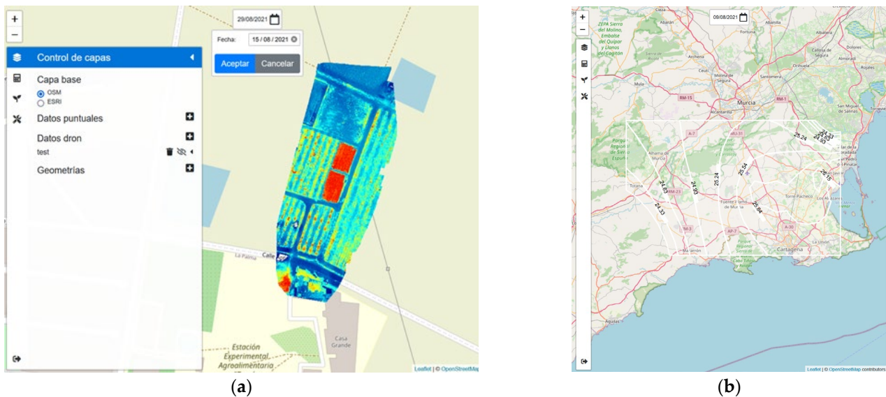
Figure 5. Detail of several functionalities found in the GIS tool. (a) Representation of a map with an information layer that contains data calculated from images collected by a drone in a specific interval of time. (b) Isoline map that cartographically shows temperature data.
