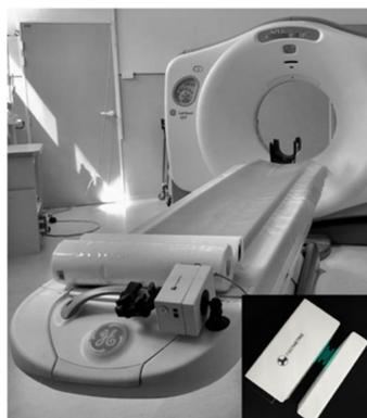
**Figure 1.** IVISCAN<sup>®</sup> dosemeter installed on a CT scan. Illustration at the bottom right shows the photometer and the induction charging station.
