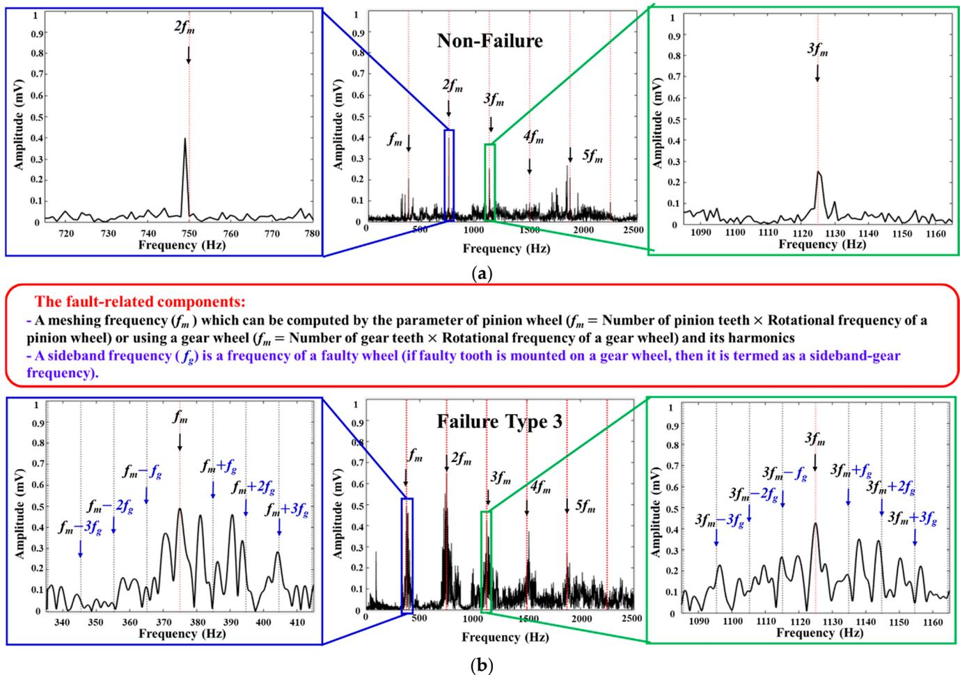
**Figure 4.** The frequency spectrum analysis of vibration samples acquired from the non-failure (a) and failure type 3 (b) conditions at 900 RPM.
