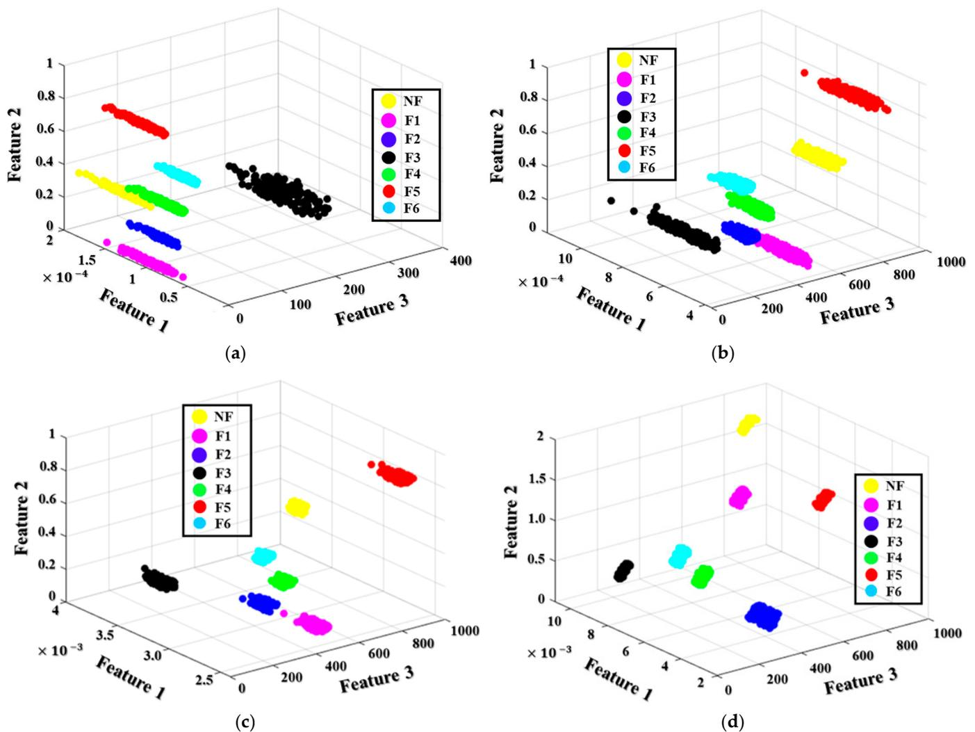
**Figure 9.** Three-dimensional visualization of samples of the seven failure types under four rotational speeds: (a) 300 RPM, (b) 600 RPM, (c) 900 RPM, and (d) 1200 RPM.
