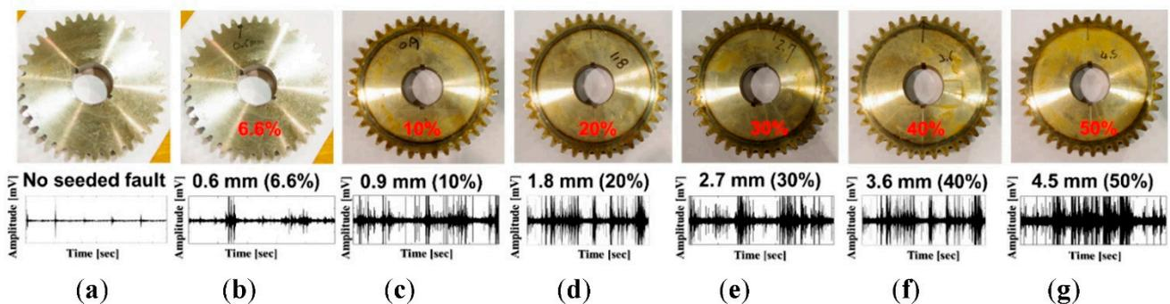
Figure 3. The multi-degree tooth cut failures of the gear wheel and the vibration signals at 600 RPM: (a) NF, (b) F1, (c) F2, (d) F3, (e) F4, (f) F5, and (g) F6.
