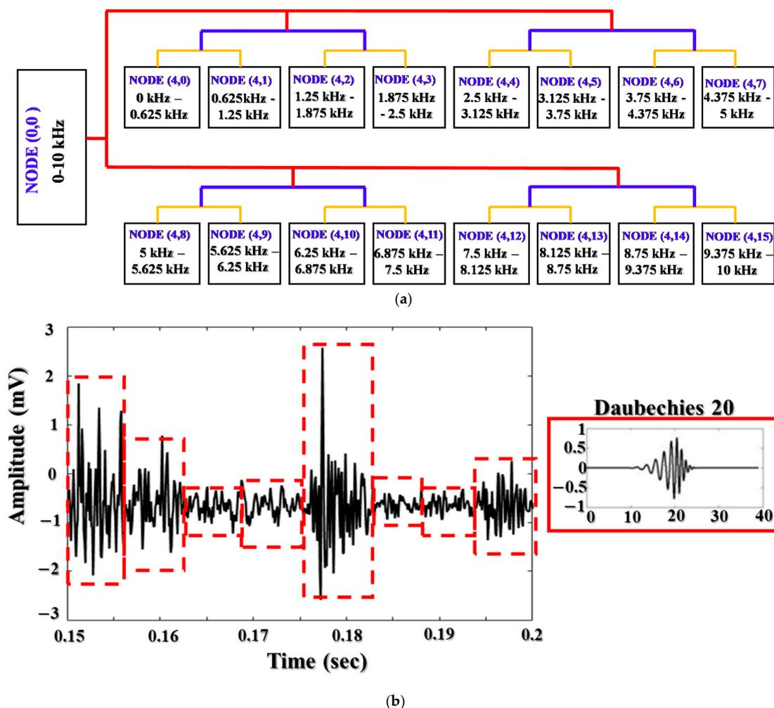
Figure 7. Four-level wavelet package decomposition (a) and the analogous oscillation patterns of a vibration signal and the Daubechies 20 function (b).
