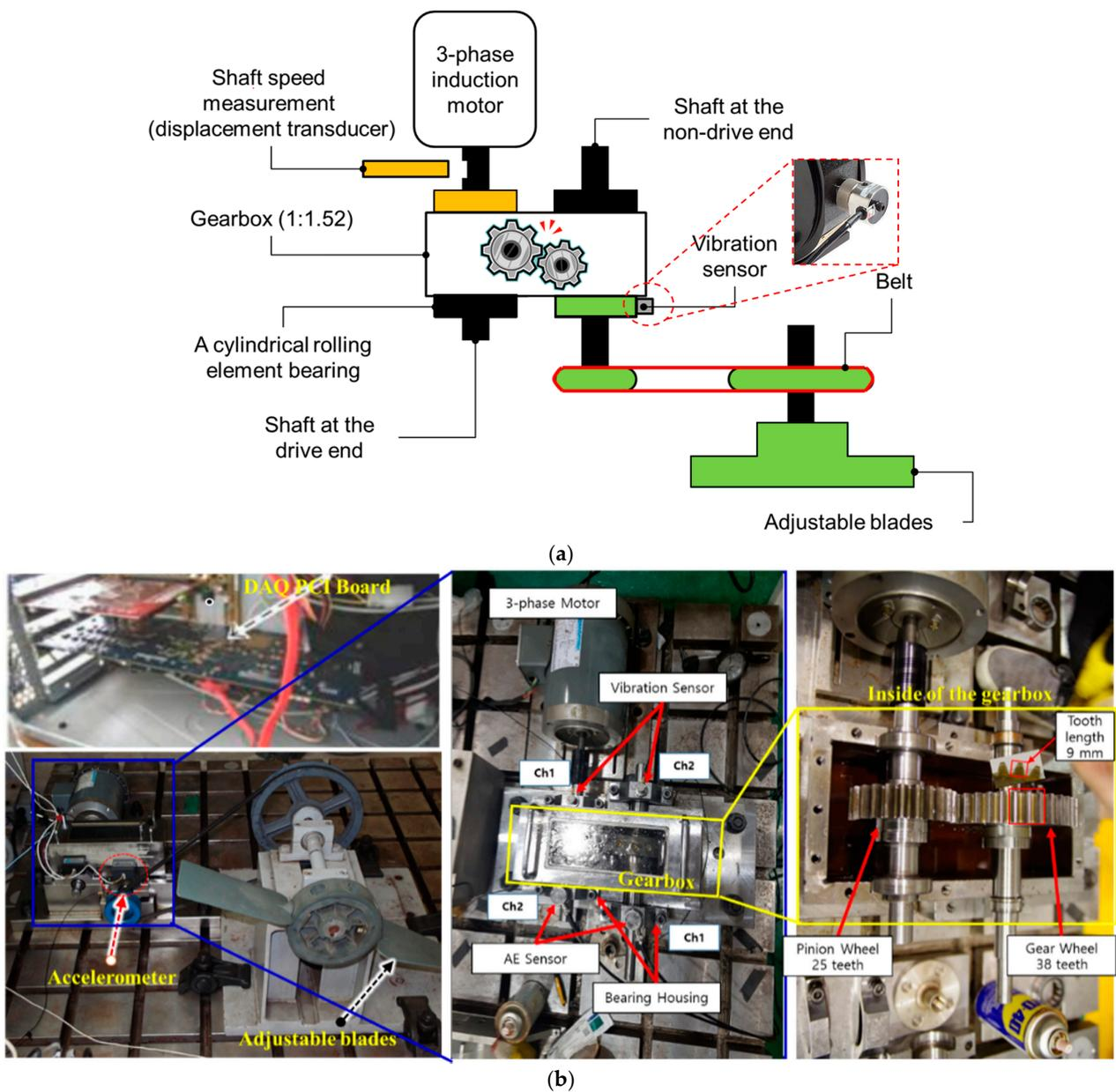
Figure 2. The experimental gearbox test rig: (a) functional structure block diagram and (b) actual arrangement of the test rig.
