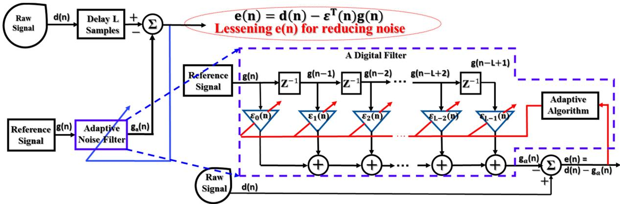
Figure 1. The functional structure of an adaptive noise filtering technique.
