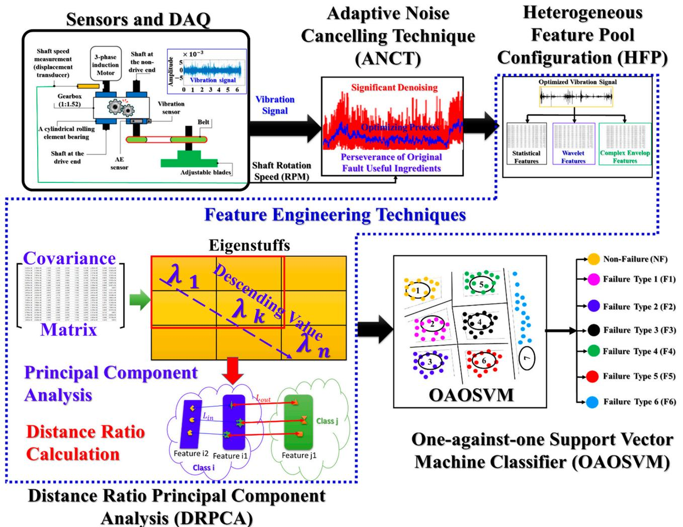
Figure 5. The processing flow and functional blocks in the proposed gearbox fault diagnosis method.
