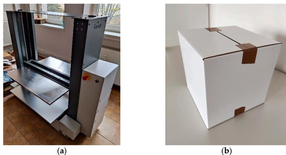
**Figure 5.** Box compression test: (a) the testing machine and (b) the box sample.
