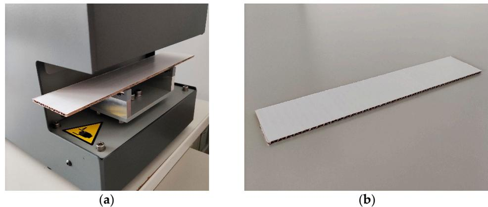
**Figure 4.** Bending stiffness test: (a) the testing socket and (b) the corrugated board sample.
