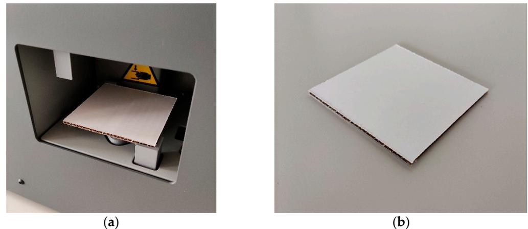
**Figure 2.** Shear stiffness test: (a) the testing socket and (b) the corrugated board sample.
