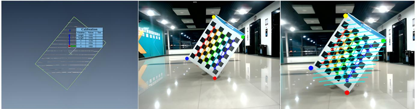
**Figure 6.** The coordinate system calibration of the multi-source sensors.
