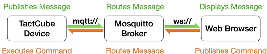
Figure 10. The two-way communications employed in the solution.
