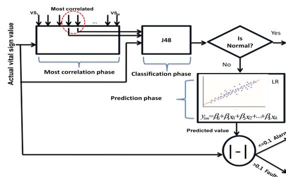
Figure 3. Our fault detection system in WBANs.
