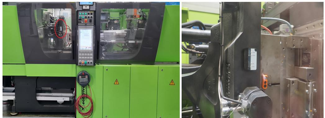
**Figure 1.** The left image shows an injection molding machine with a mounted 3-axis accelerometer (sensor marked by a red circle in the center of the image). The right picture shows the mounting of the same sensor in detail.
