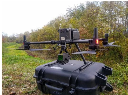
**Figure 8.** DJI Matrice 300 RTK with DJI Zenmuse L1 ALS.
