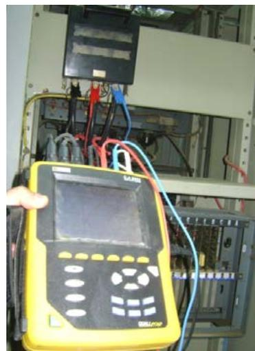
Figure 17. Power quality phenomena measurements using C.A 8334B.
