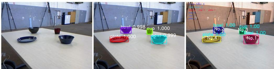
**Figure 4.** The detection results of freiburg2\_dishes using self-training weight. From left to right, the first image is the original RGB image. The second is the detection result of Mask R-CNN. The third is the detection result of Mask R-CNN with Deepsort.
