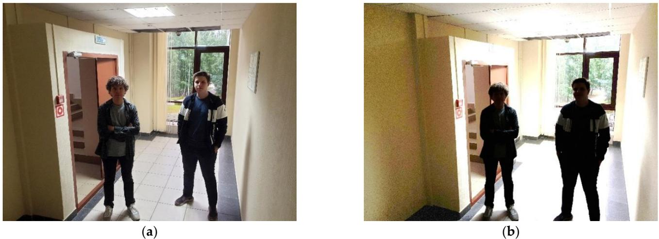
Figure 5. Highlights in the camera image: (a) WDR on; (b) WDR off.
