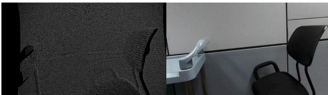
**Figure 3.** Holes in the reprojected depth map and corresponding color image.
