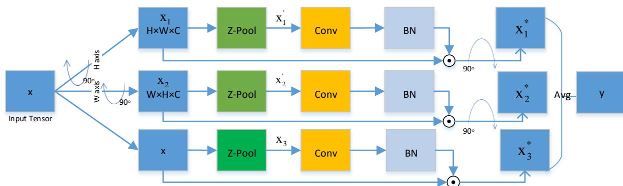
**Figure 5.** Illustration of the architecture of the convolutional triple attention module (CTAM).
