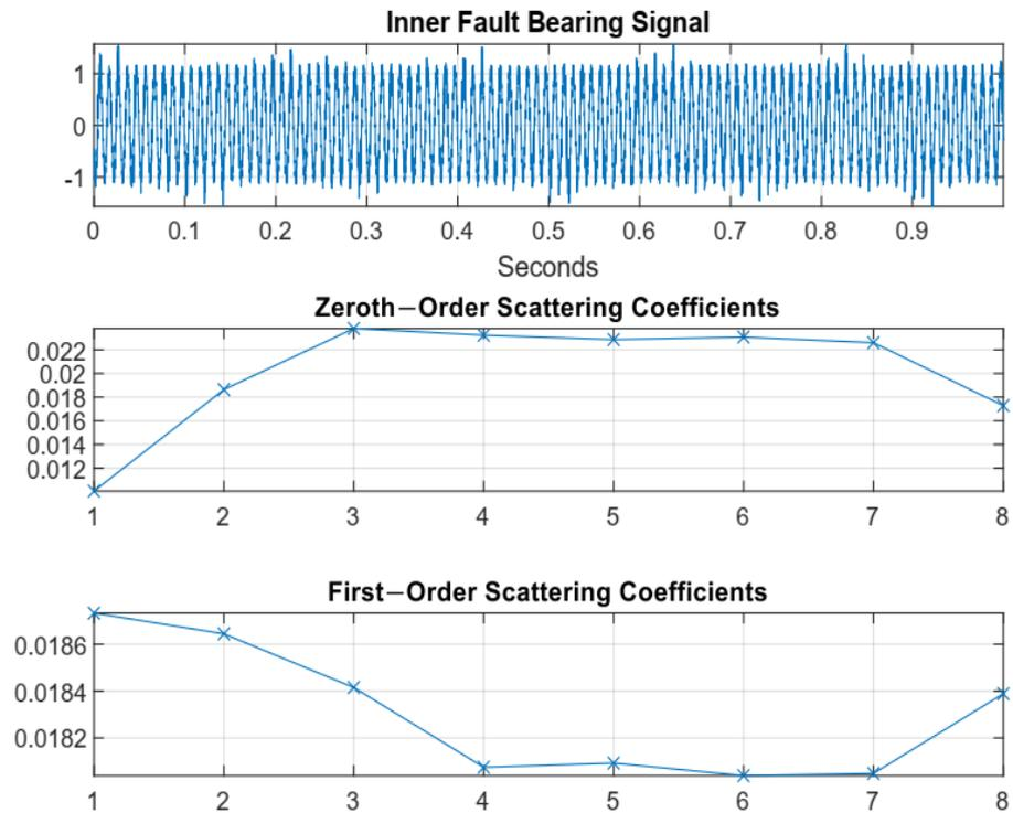
**Figure 8.** Time series bearing data, 0th and 1st order scattering coefficients of the inner race faulty conditions.
