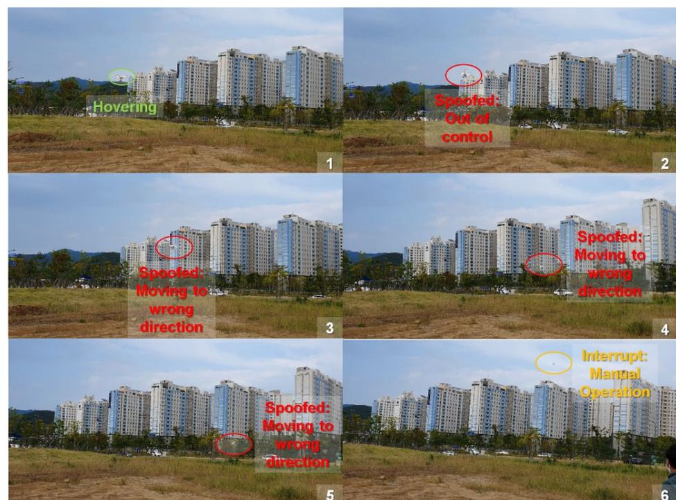
**Figure 12.** Spoofed DJI Phantom in the flight test.
