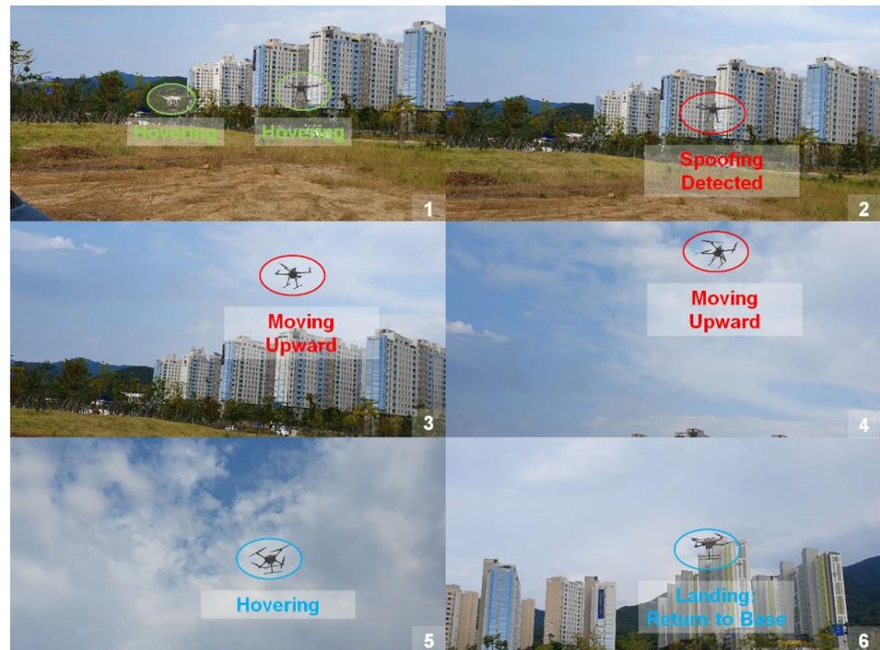
**Figure 15.** Spoofing detection and emergency landing of our drone in the flight test.
