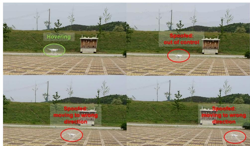
**Figure 8.** Test result of the Phantom drone.
