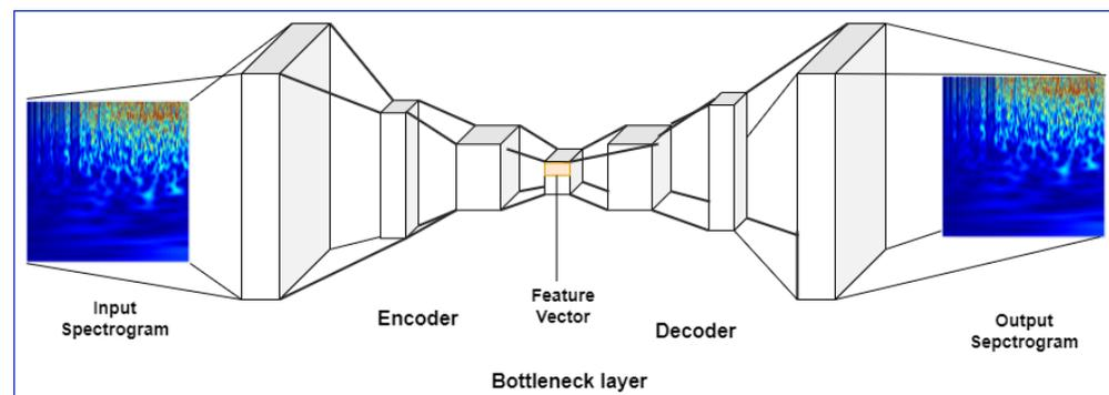
**Figure 3.** Visualization of the proposed architecture of stacked autoencoder.
