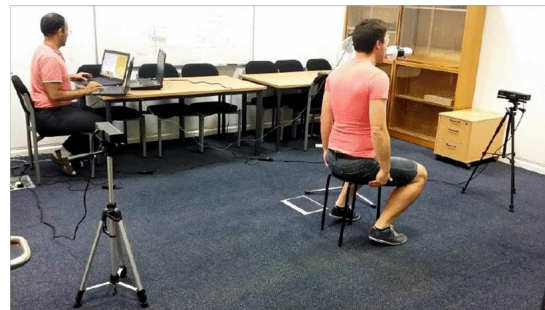
Figure 3. Measurement setup with two Kinect v2 cameras facing each other. The subject sits on a chair without a backrest and breathes through a reference spirometer. The image is taken from [43], licensed via Creative Commons License, and not changed for this work.
